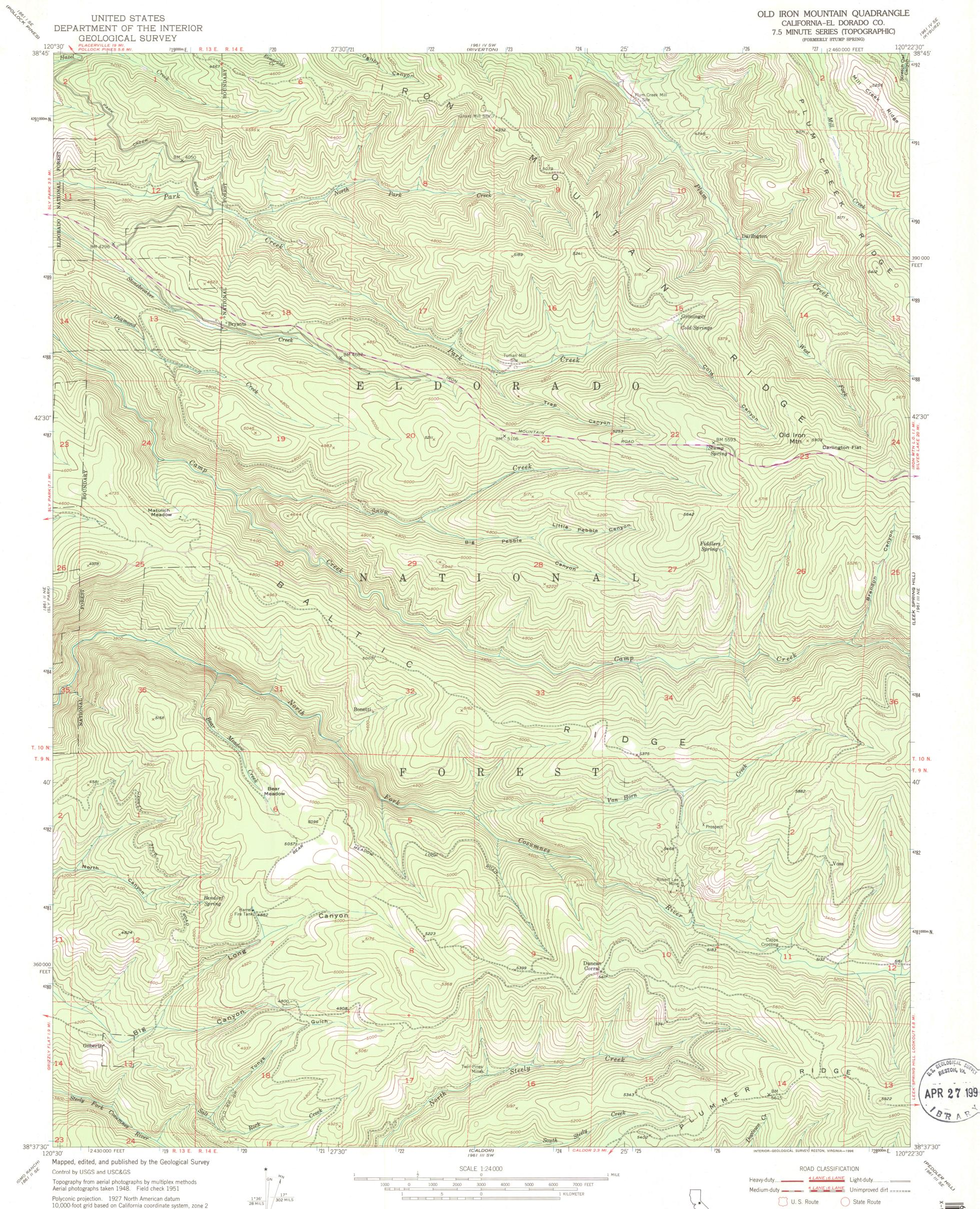
Polyconic projection. 1927 North American datum 10,000-foot grid based on California coordinate system, zone 2 1000-meter Universal Transverse Mercator grid ticks, zone 10, shown in blue To place on the predicted North American Datum 1983 move the projection lines 14 meters north and 89 meters east as shown by dashed corner ticks
