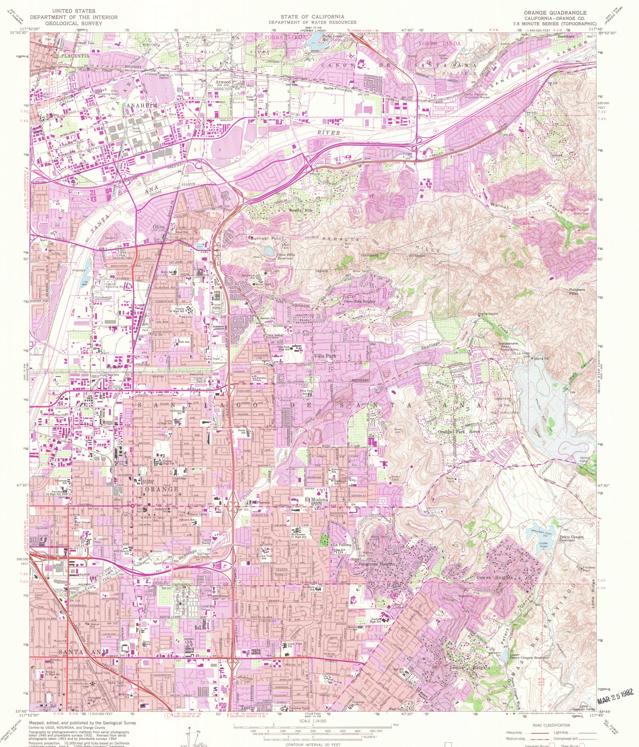
Polyconic projection. 10,000-foot grid ticks based on California coordinate system, zone 6. 1000-meter Universal Transverse Mercator grid ticks, zone 11, shown in blue. 1927 North American Datum. To place on the predicted North American Datum 1983 move the projection lines 1 meter north and 84 meters east as shown by dashed corror ticks shown by dashed corner ticks
