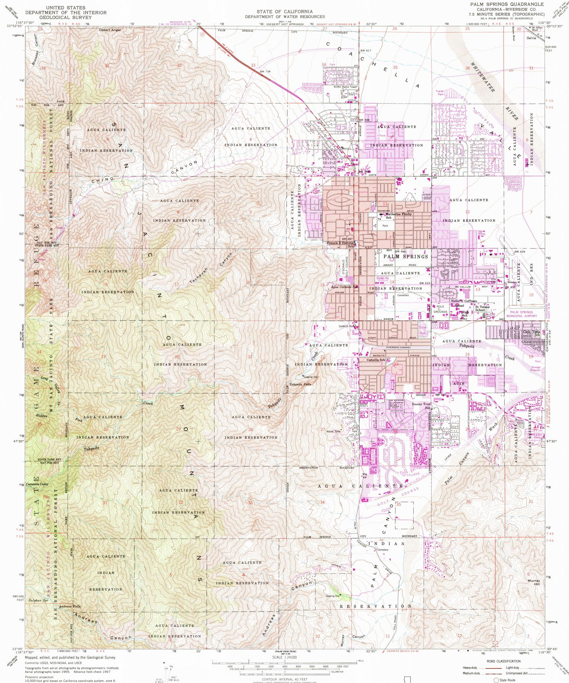
10,000-foot grid based on California coordinate system, zone 6 1000-meter Universal Transverse Mercator grid ticks, zone 11, shown in blue. 1927 North American Datum To place on the predicted North American Datum 1983 move the projection lines 80 meters east as shown by dashed corner ticks
