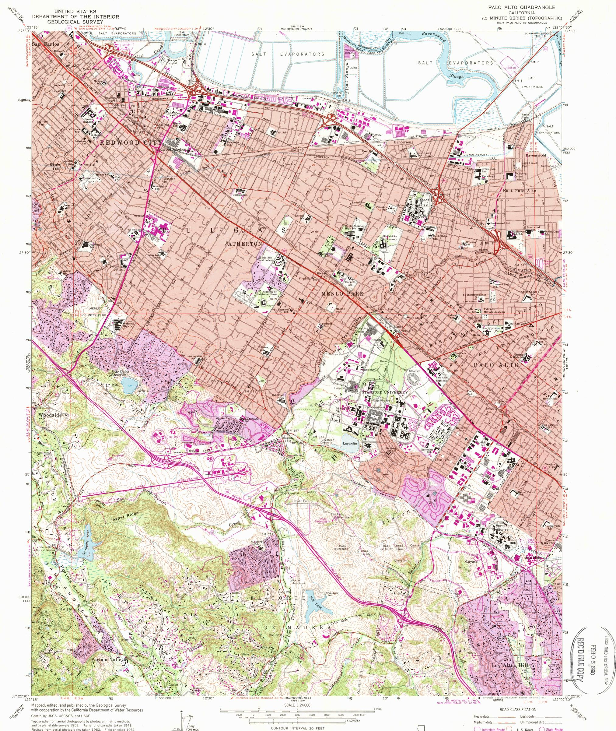
Revised from aerial photographs taken 1960. Field checked 1961 Polyconic projection. 1927 North American datum 10,000-foot grid based on California coordinate system, zone 3 1000-meter Universal Transverse Mercator grid ticks, zone 10, shown in blue Red tint indicates area in which only landmark buildings are shown
