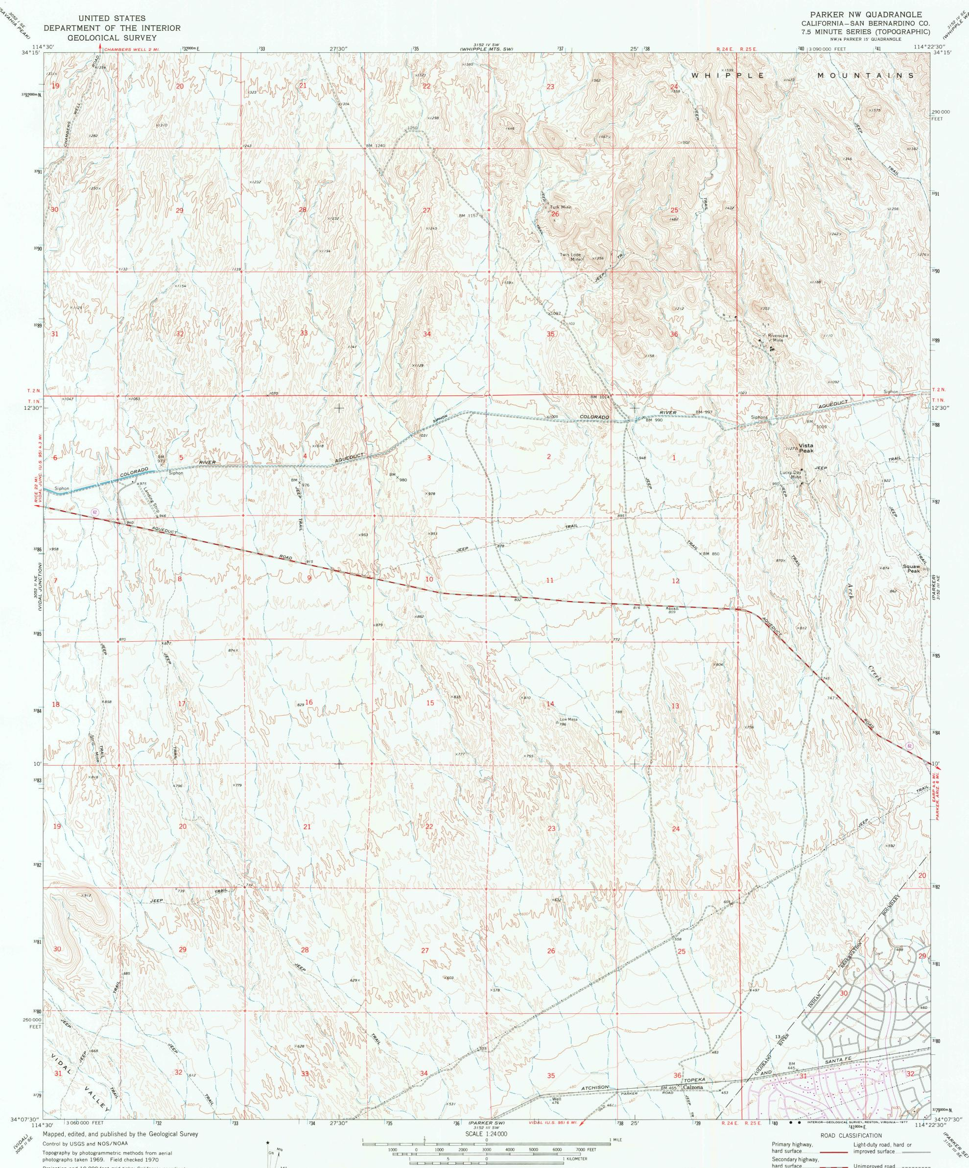
Projection and 10,000-foot grid ticks: California coordinate system, zone 5 (Lambert conformal conic) 1000-meter Universal Transverse Mercator grid ticks, zone 11, shown in blue. 1927 North American datum
