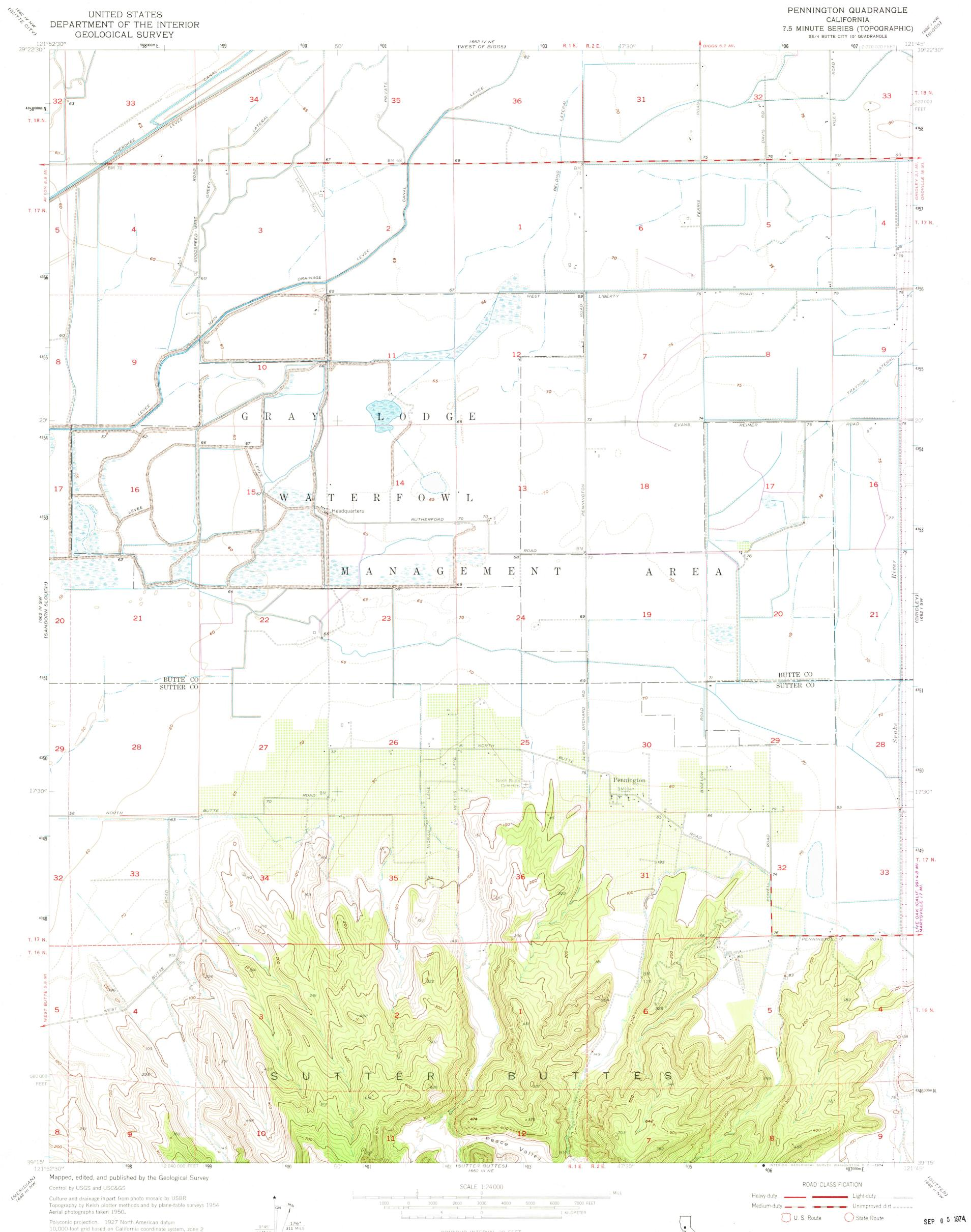
Polyconic projection. 1927 North American datum 10,000-foot grid based on California coordinate system, zone 2 Dashed land lines indicate approximate locations Unchecked elevations are shown in brown
