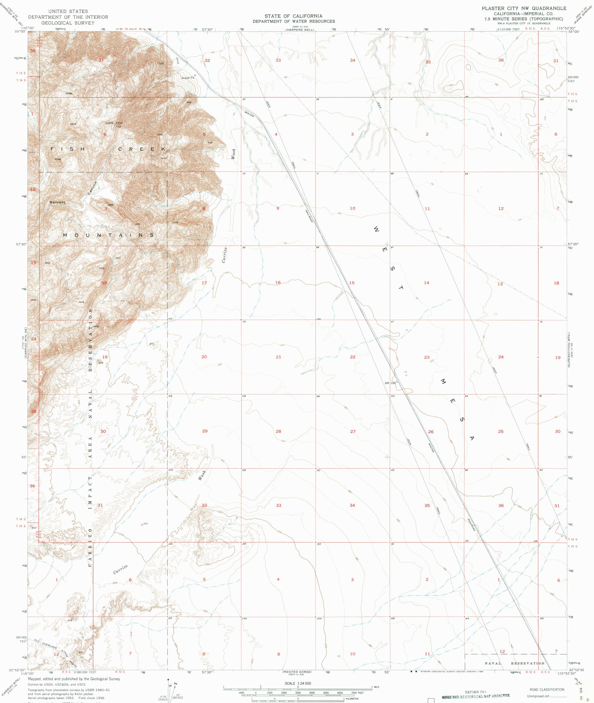
Polyconic projection. 1927 North American datum 10,000-foot grid based on California coordinate system, zone 6 1000-meter Universal Transverse Mercator grid ticks, zone 11, shown in blue To place on the predicted North American Datum 1983 move the projection lines 3 meters south and 77 meters east as shown by dashed corner ticks
