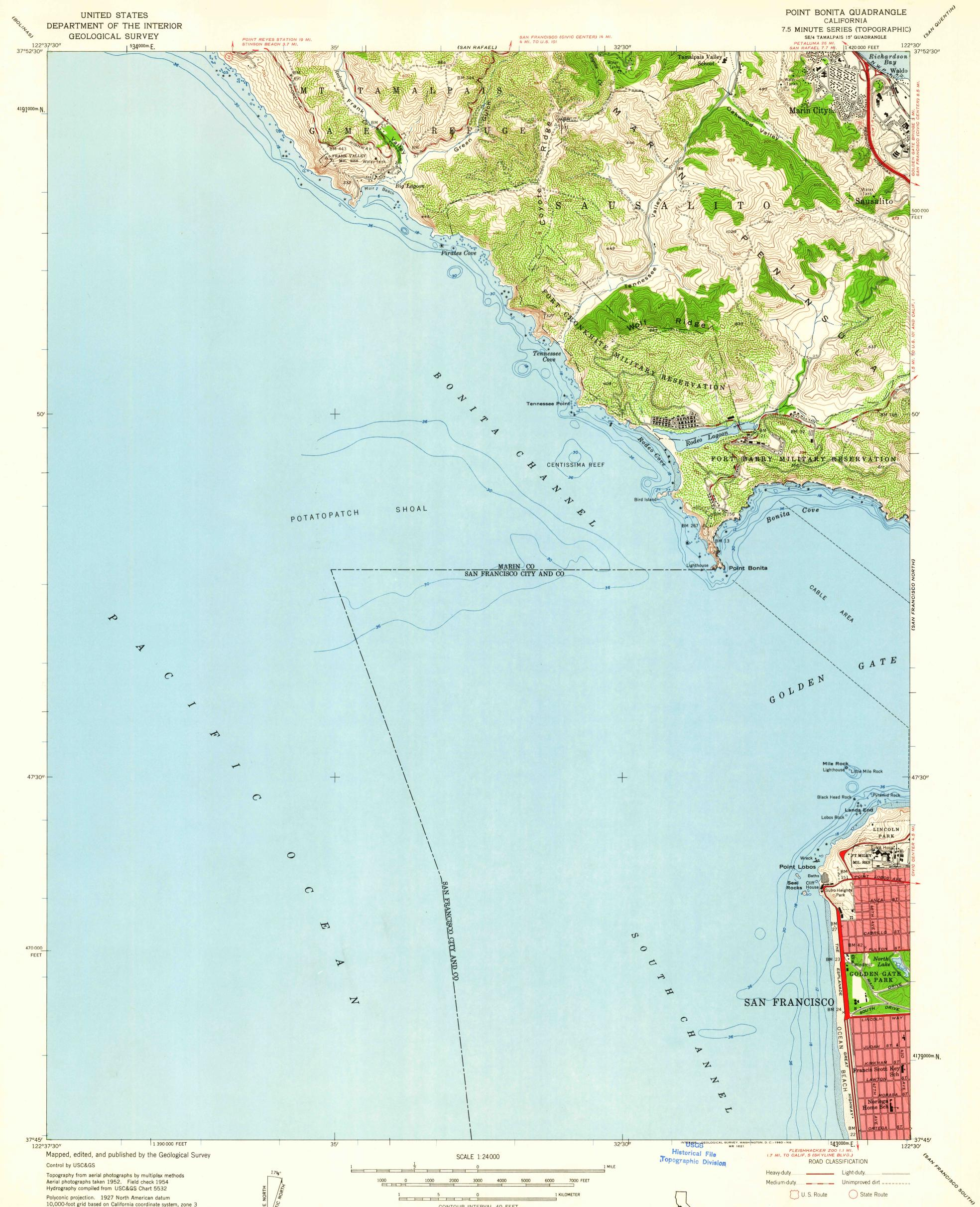
Polyconic projection. 1927 North American datum 10,000-foot grid based on California coordinate system, zone 3 Red tint indicates areas in which only landmark buildings are shown Unchecked elevations are shown in brown 1000-meter Universal Transverse Mercator grid ticks, zone 10, shown in blue
