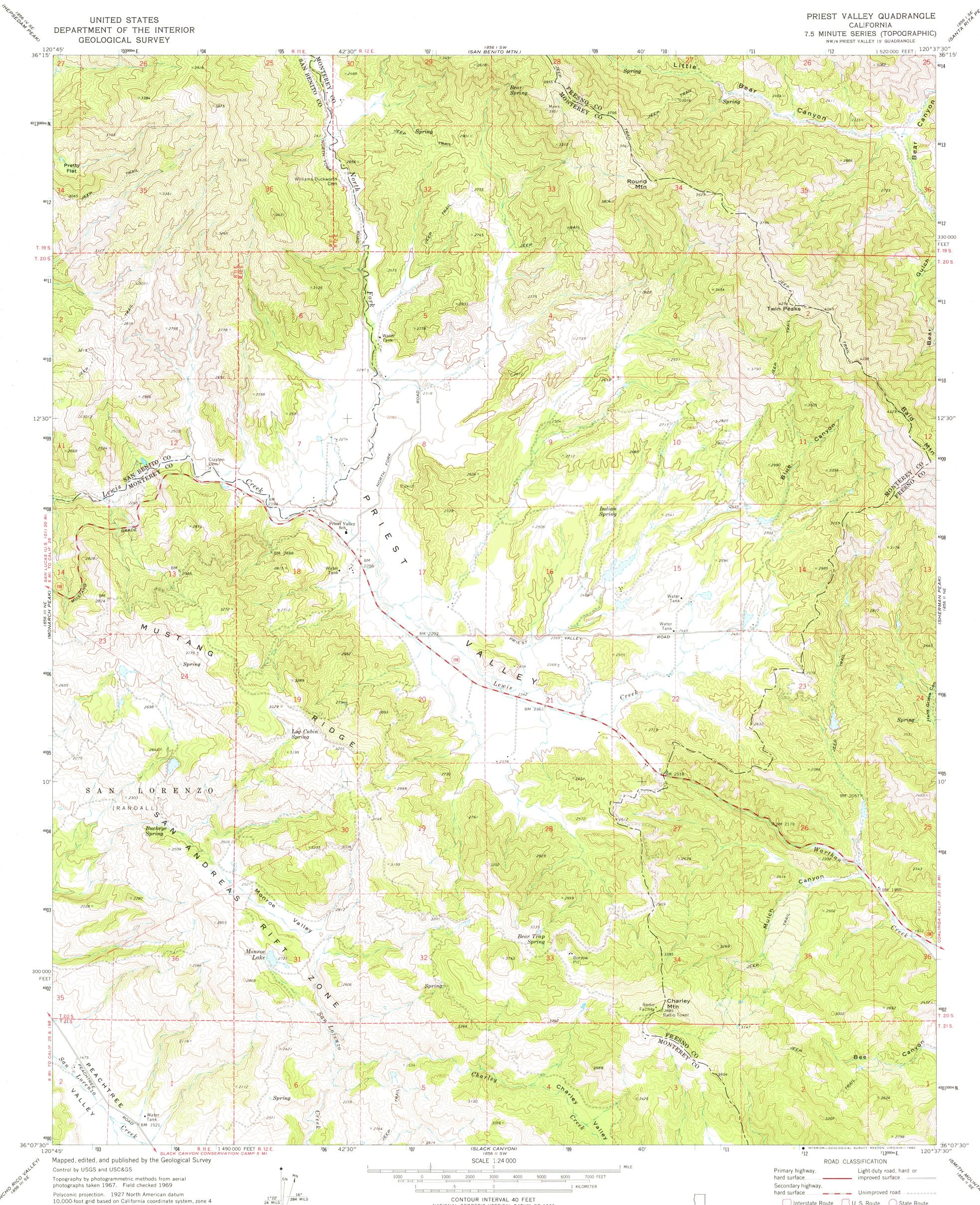
10,000-foot grid based on California coordinate system, zone 4 1000-meter Universal Transverse Mercator grid ticks, zone 10, shown in blue To place on the predicted North American Datum 1983 move the projection lines 8 meters north and 90 meters east as shown by dashed corner ticks
