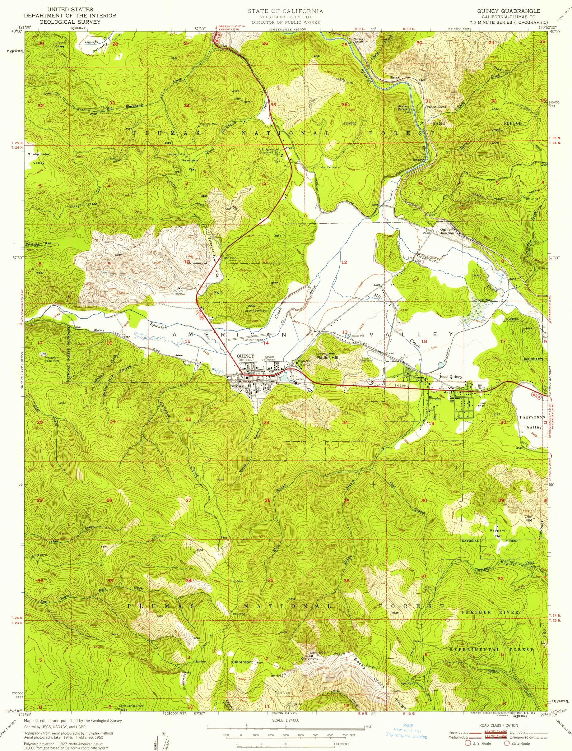
Polyconic projection. 1927 North American datum 10,000-foot grid based on California coordinate system, zone 1 Dashed land lines indicate approximate location Unchecked elevations are shown in brown 1000-meter Universal Transverse Mercator grid ticks, zone 10, shown in blue
