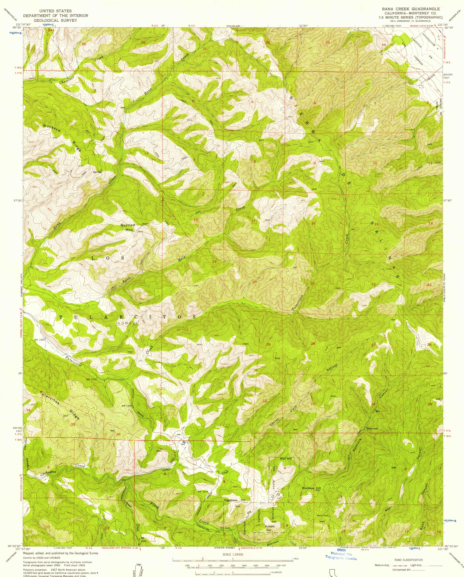
Polyconic projection. 1927 North American datum 10,000-foot grid based on California coordinate system, zone 4 1000-meter Universal Transverse Mercator grid ticks, zone 10, shown in blue
