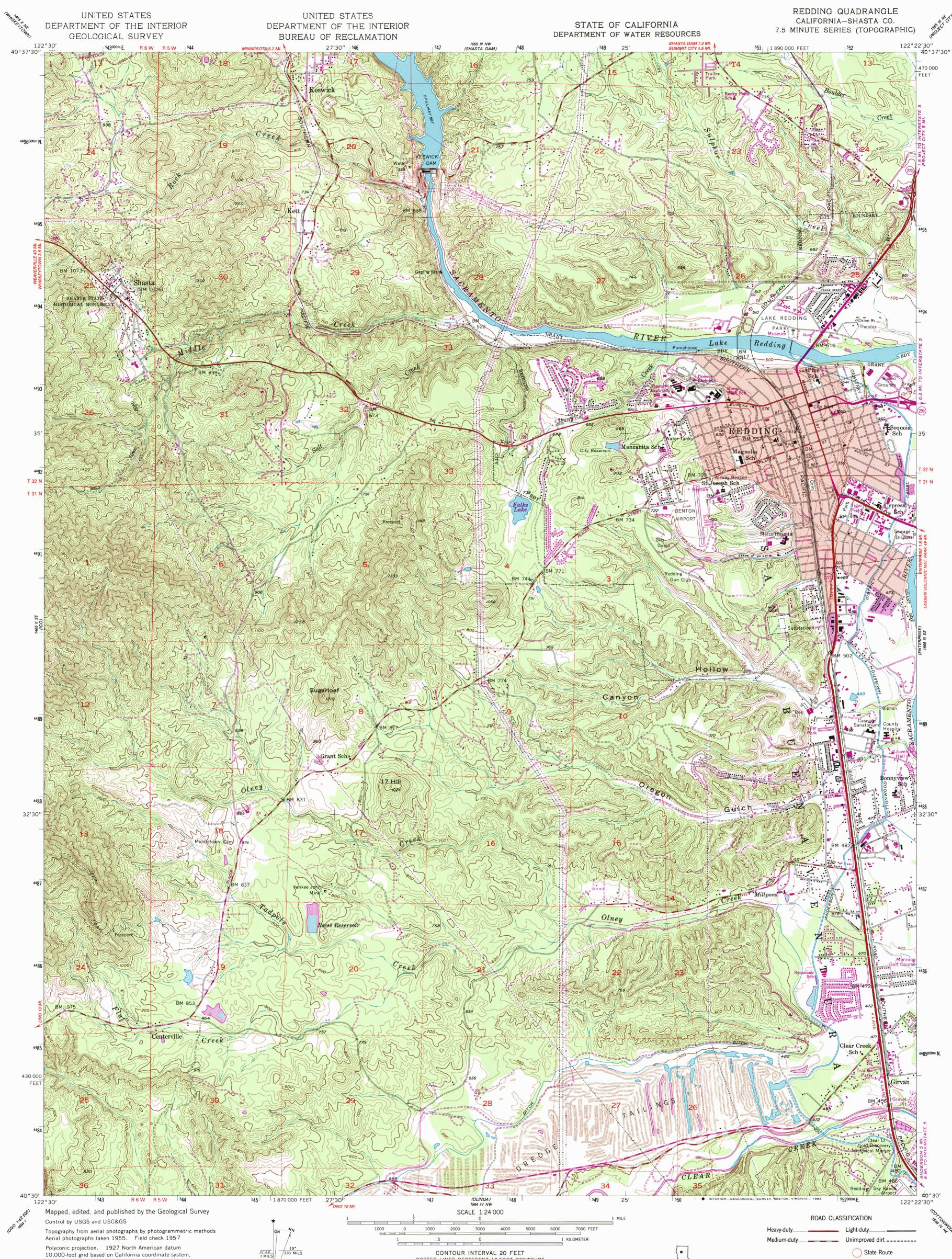
10,000-foot grid based on California coordinate system, zone 1 1000-meter Universal Transverse Mercator grid ticks, zone 10, shown in blue UTM GRID AND 1969 MAGNETIC NORTH DECLINATION AT CENTER OF SHEET To place on the predicted North American Datum 1983 move the projection lines 18 meters north and 93 meters east as shown by dashed corner ticks Red tint indicates areas in which only landmark buildings are shown
