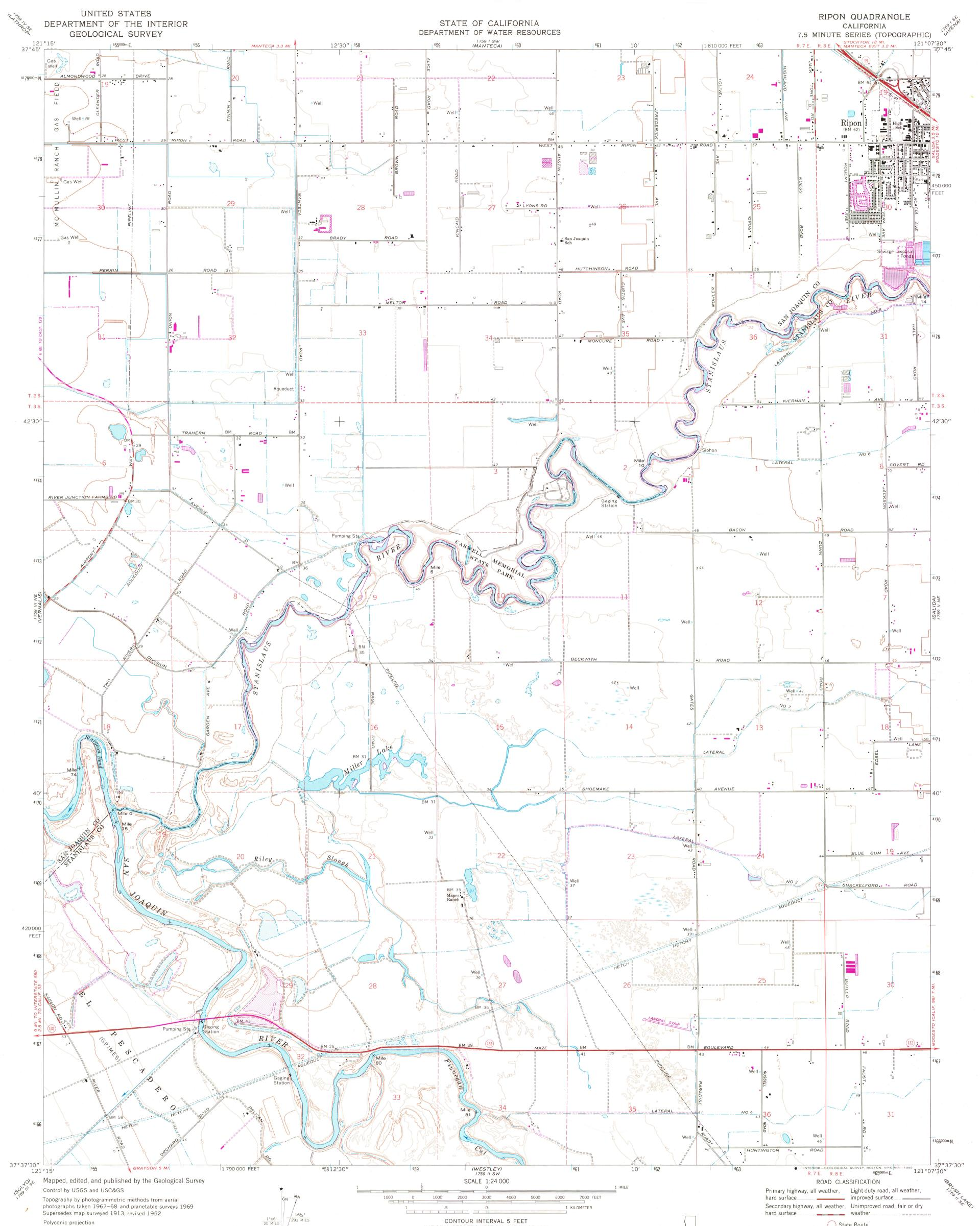
Polyconic projection 10,000-foot grid based on California coordinate system, zone 3 1000-meter Universal Transverse Mercator grid ticks, zone 10, shown in blue. 1927 North American Datum To place on the predicted North American Datum 1983 move the projection lines 12 meters north and 92 meters east as shown by dashed corner ticks There may be private inholdings within the boundaries
