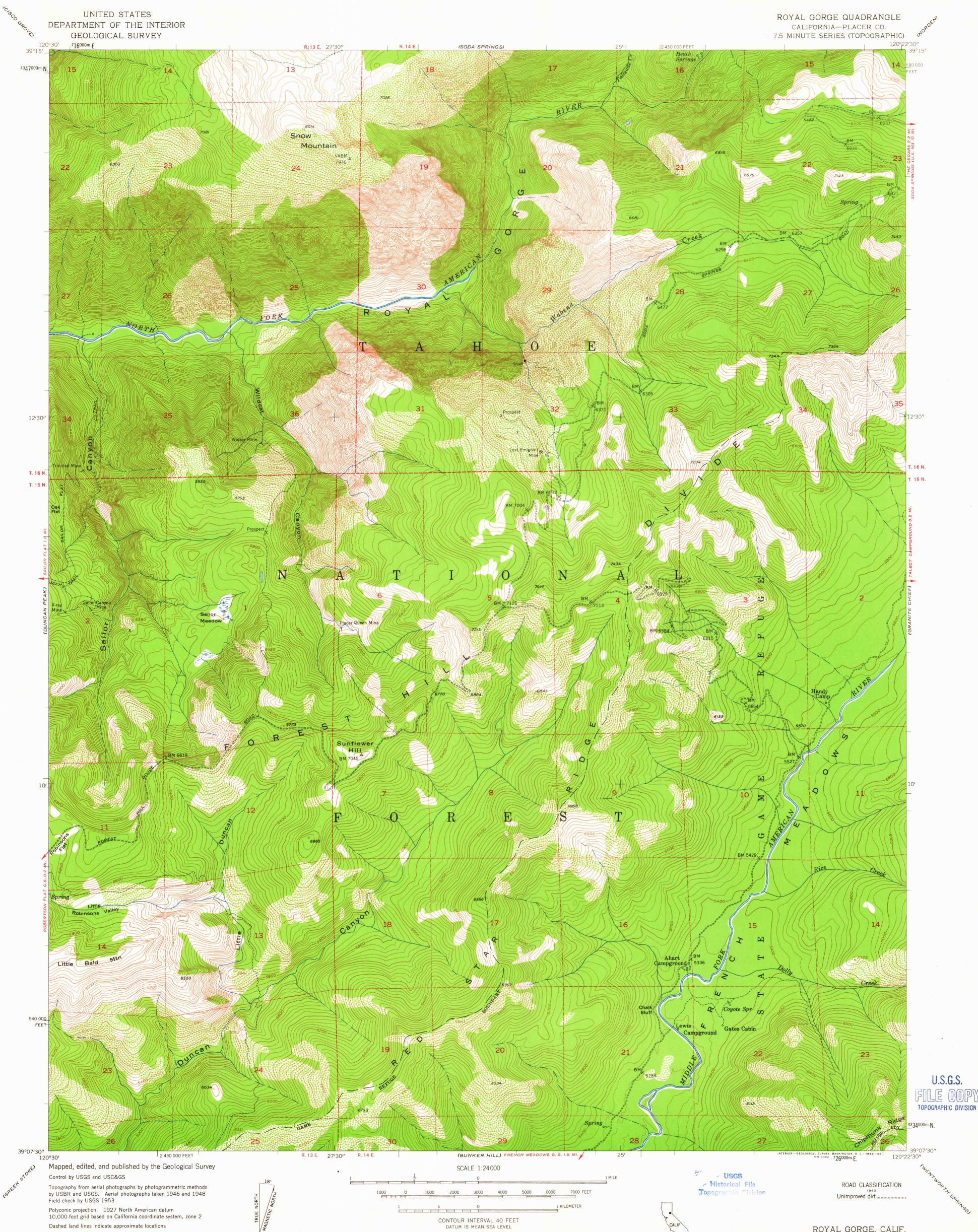
Polyconic projection. 1927 North American datum 10,000-foot grid based on California coordinate system, zone 2 Dashed land lines indicate approximate locations Unchecked elevations are shown in brown 1000-meter Universal Transverse Mercator grid ticks, zone 10, shown in blue
