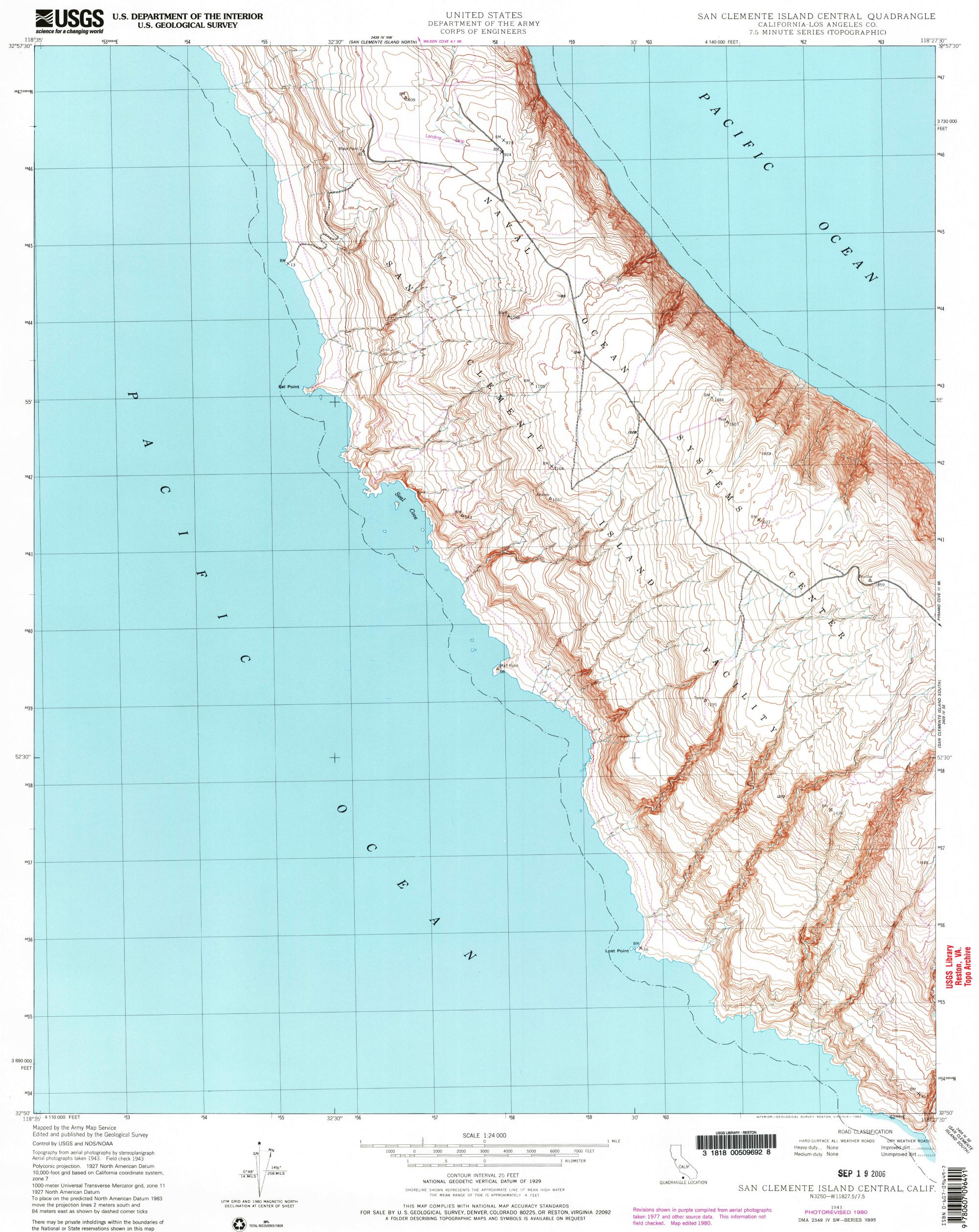
Polyconic projection. 1927 North American Datum 10,000-foot grid based on California coordinate system, zone 7 1000-meter Universal Transverse Mercator grid, zone 11 1927 North American Datum To place on the predicted North American Datum 1983 move the projection lines 2 meters south and 84 meters east as shown by dashed corner ticks
