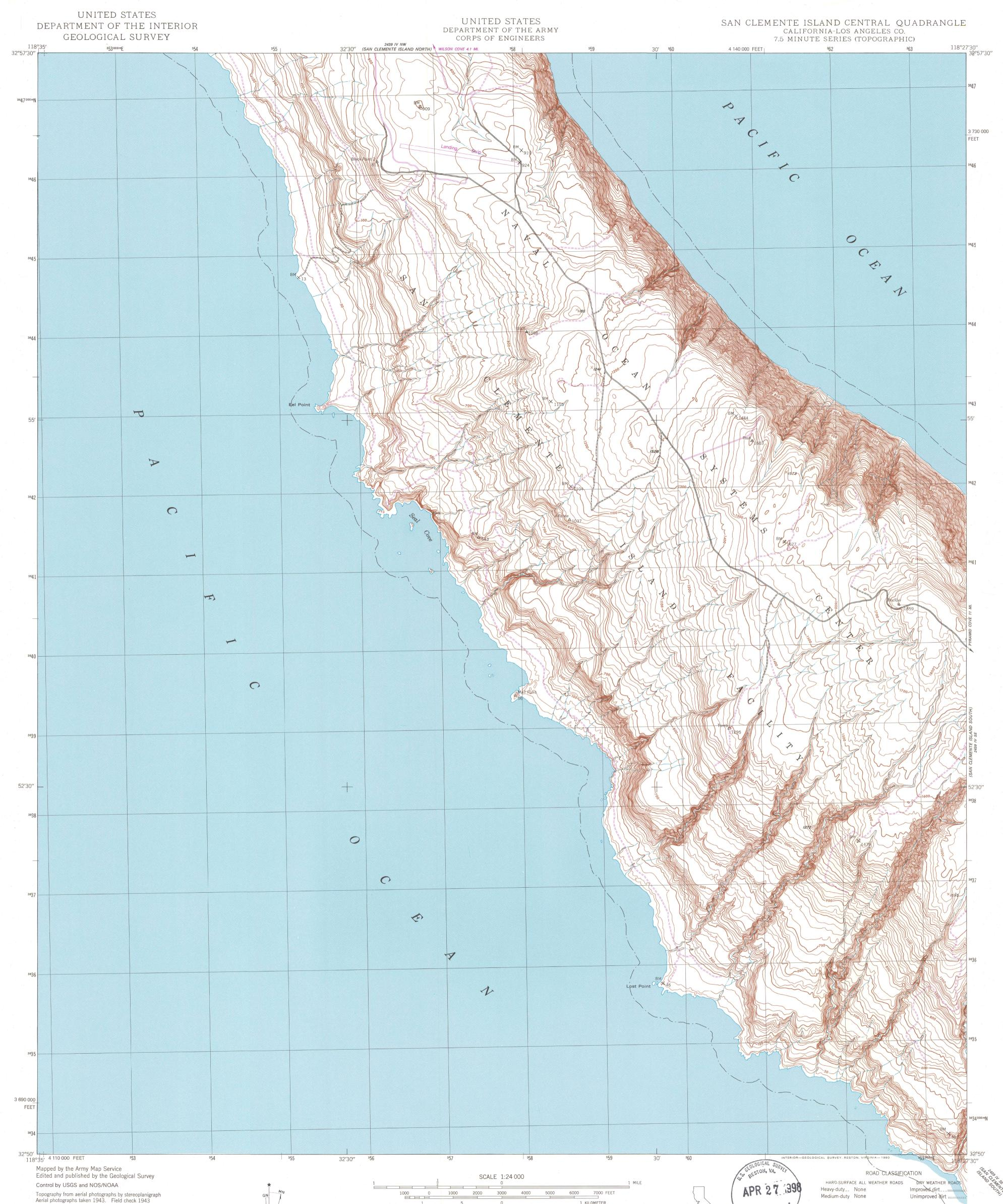
Polyconic projection. 1927 North American Datum 10,000-foot grid based on California coordinate system, zone 7 1000-meter Universal Transverse Mercator grid, zone 11 1927 North American Datum To place on the predicted North American Datum 1983 move the projection lines 2 meters south and 84 meters east as shown by dashed corner ticks
