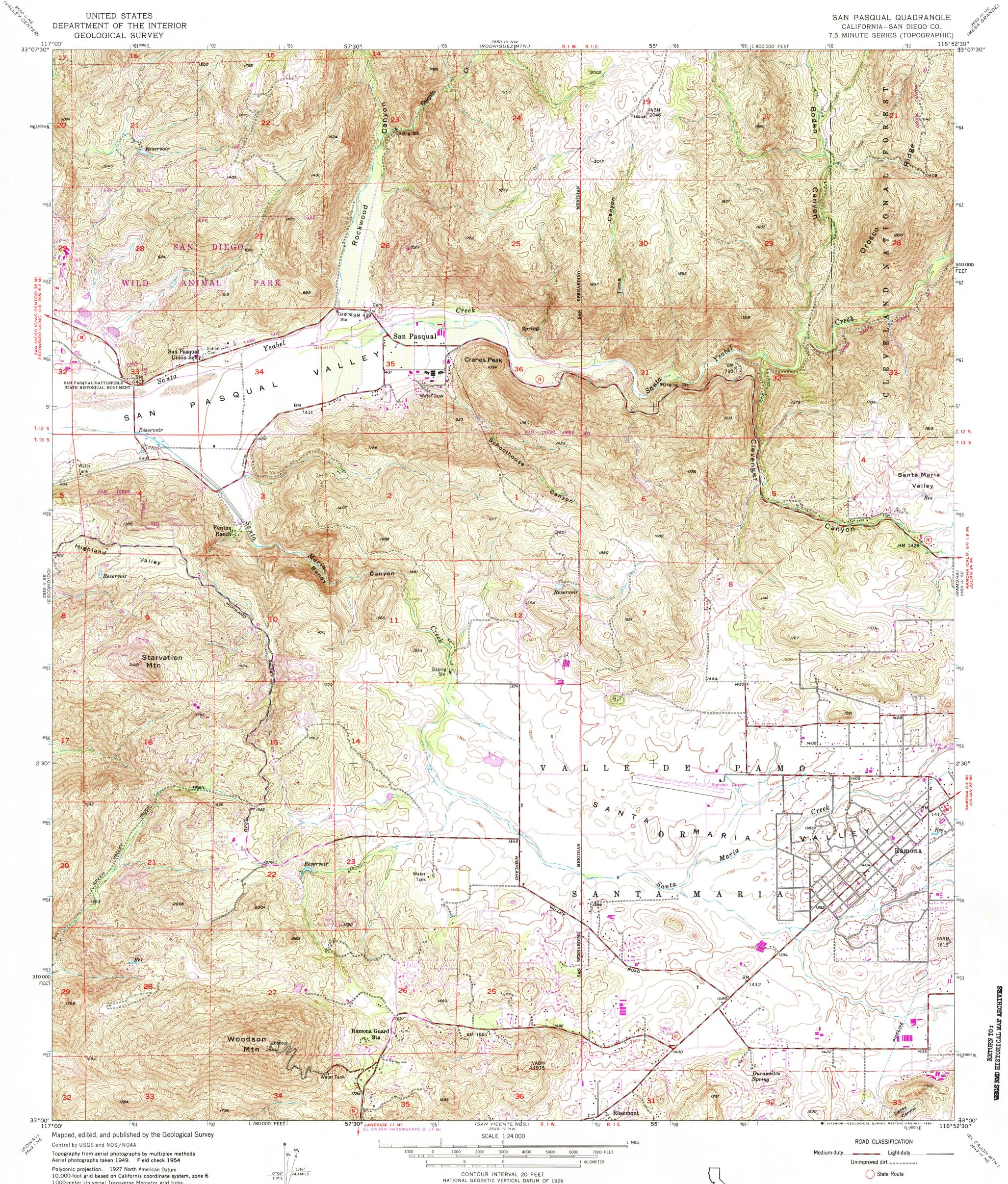
1000-meter Universal Transverse Mercator grid ticks, zone 11, shown in blue To place on the predicted North American Datum 1983, move the projection lines 2 meters south and 80 meters east as shown by dashed corner ticks
