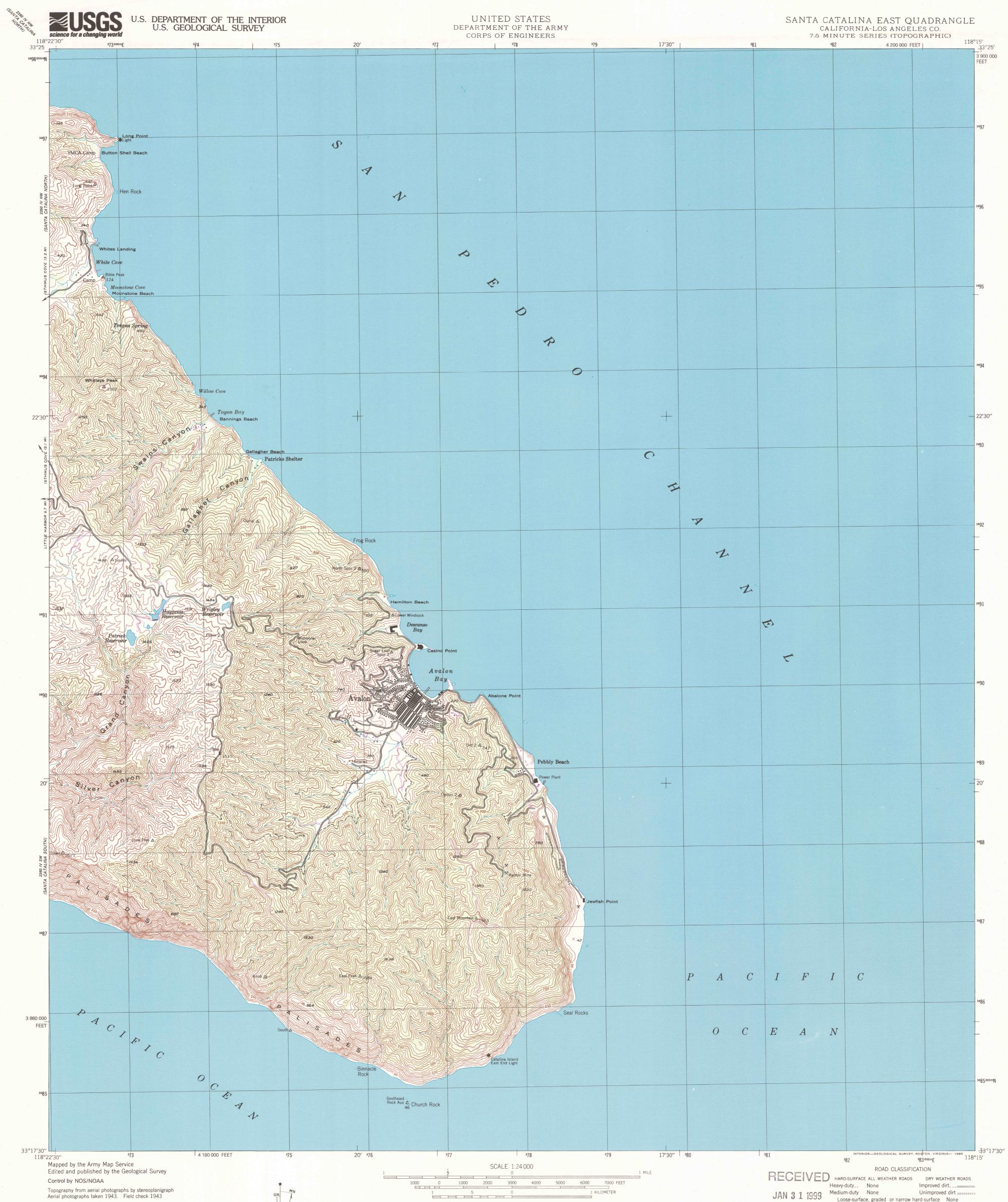
Polyconic projection. 1927 North American datum 10,000-foot grid based on California coordinate system, zone 7 1000-meter Universal Transverse Mercator grid, zone 11 To place on the predicted North American Datum 1983 move the projection lines 0 meters north and 84 meters east as shown by dashed corner ticks
