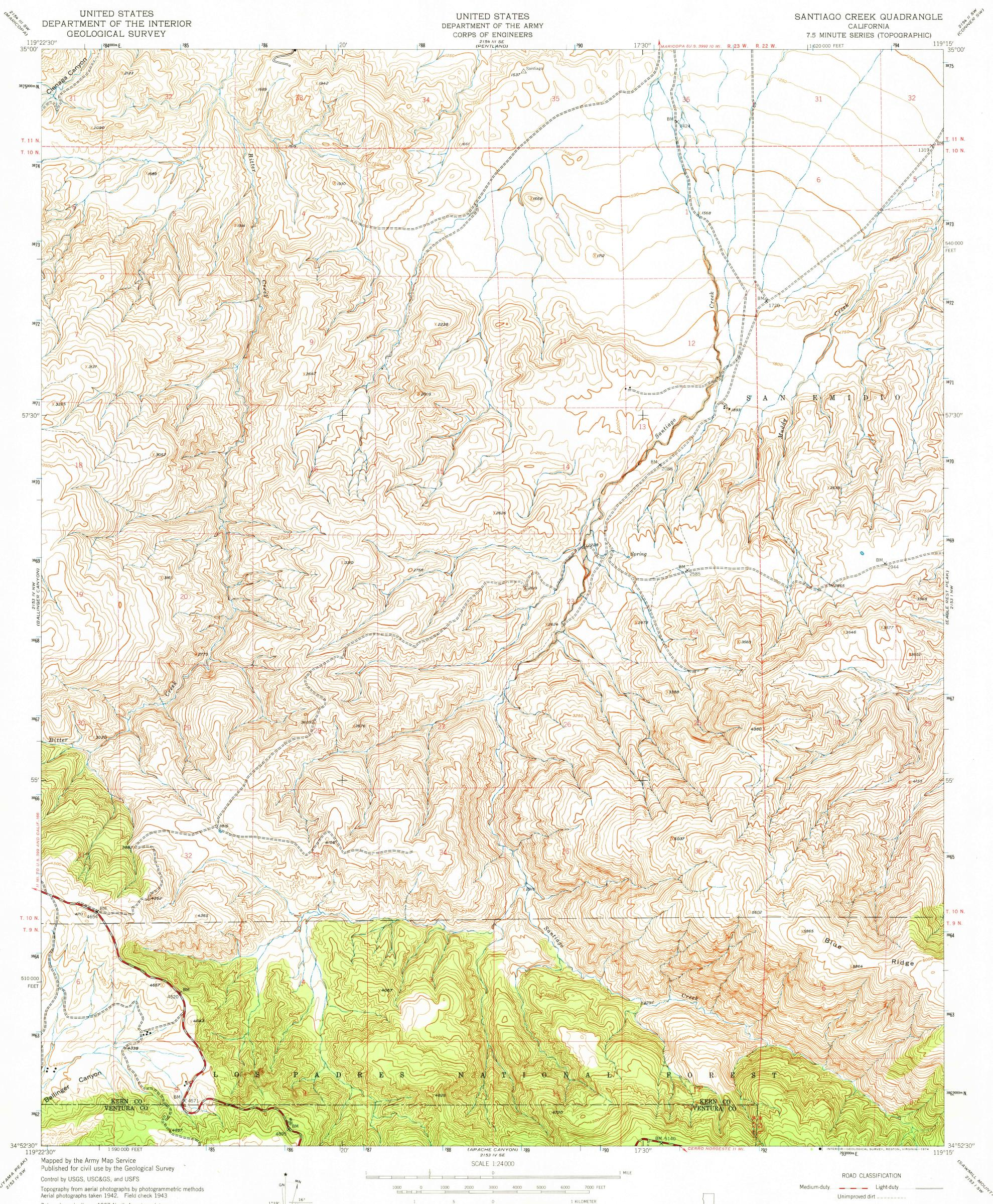
Polyconic projection. 1927 North American datum 10,000-foot grid based on California coordinate system, zone 5 1000-meter Universal Transverse Mercator grid ticks, zone 11, shown in blue
