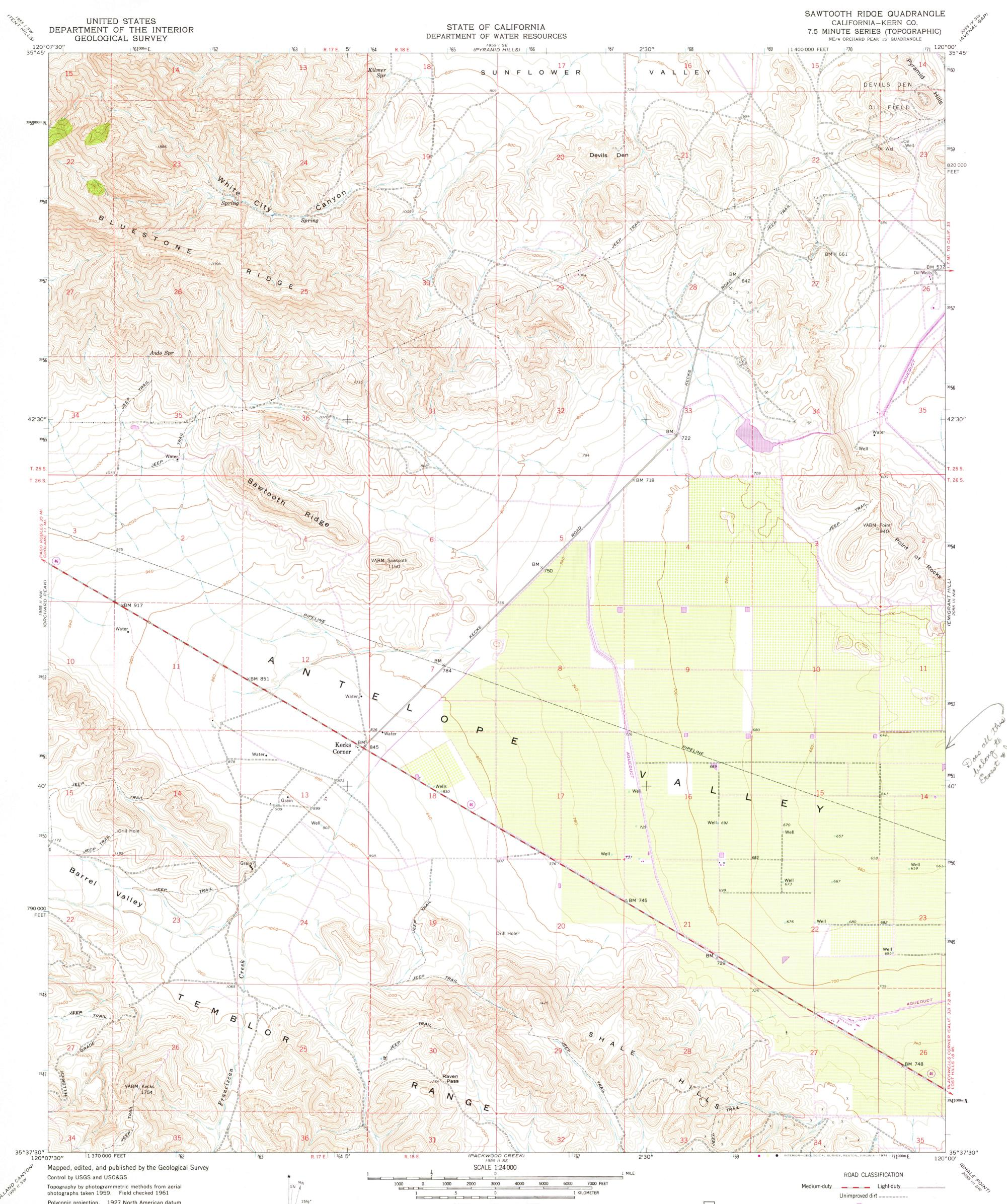
Polyconic projection. 1927 North American datum 10,000-foot grid based on California coordinate system, zone 5 1000-meter Universal Transverse Mercator grid ticks, zone 10, shown in blue
