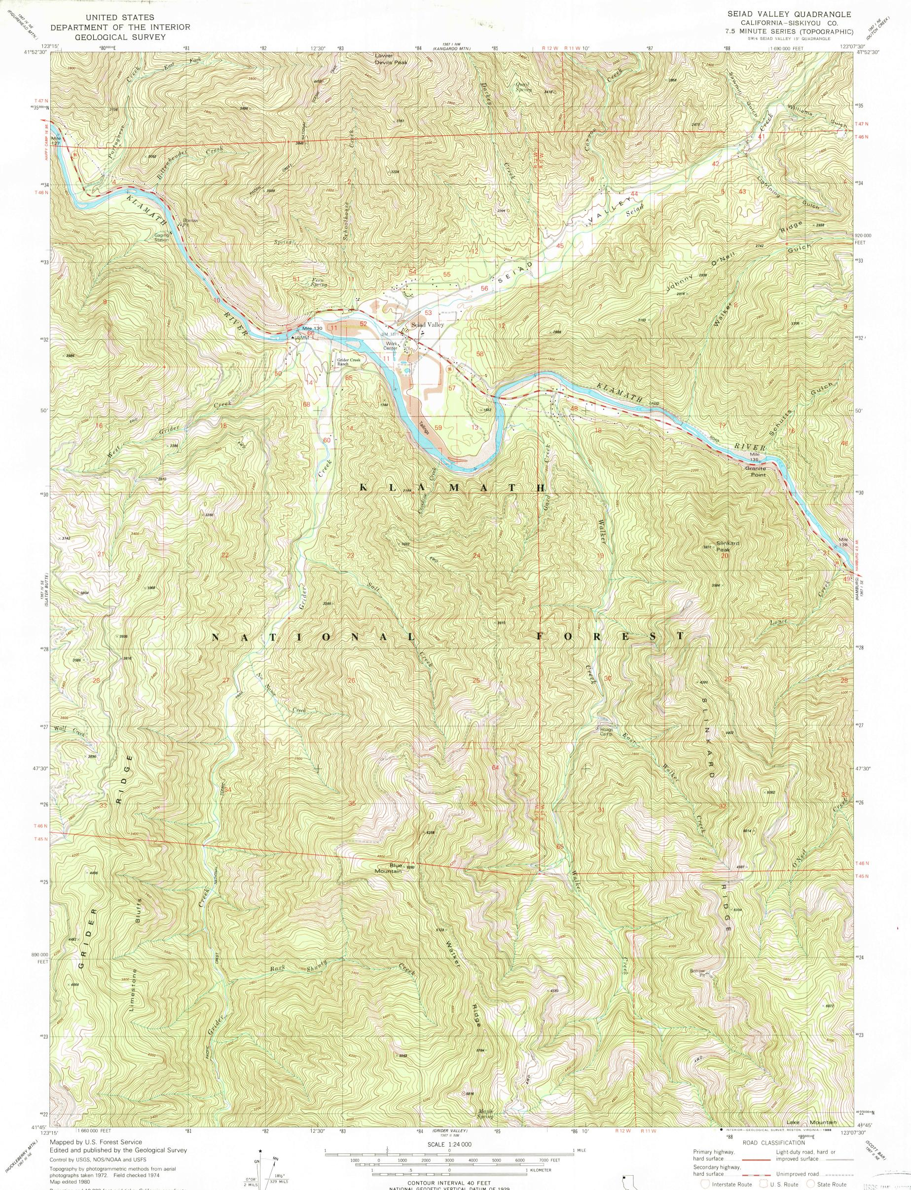
Projection and 10,000-foot grid ticks: California coordinate system, zone 1 (Lambert conformal conic) 1000-meter Universal Transverse Mercator grid, zone 10 1927 North American Datum To place on the predicted North American Datum 1983 move the projection lines 20 meters north and 95 meters east as shown by dashed corner ticks Certain land lines are not shown because of insufficient data
