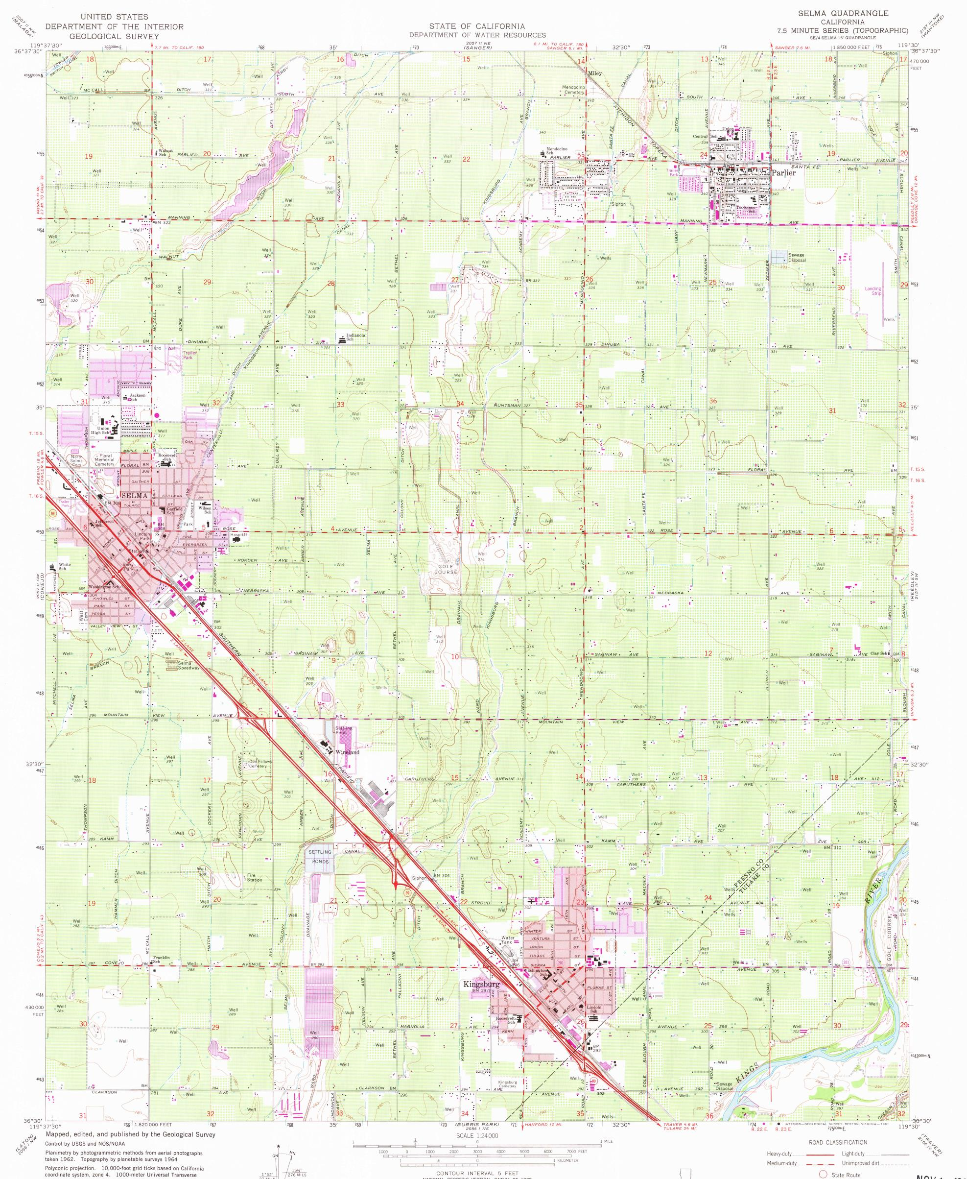
coordinate system, zone 4. 1000-meter Universal Transverse Mercator grid ticks, zone 11, shown in blue. 1927 North American Datum. To place on the predicted North American Datum 1983 move the projection lines 8 meters north and 87 meters east as shown by dashed corner ticks
