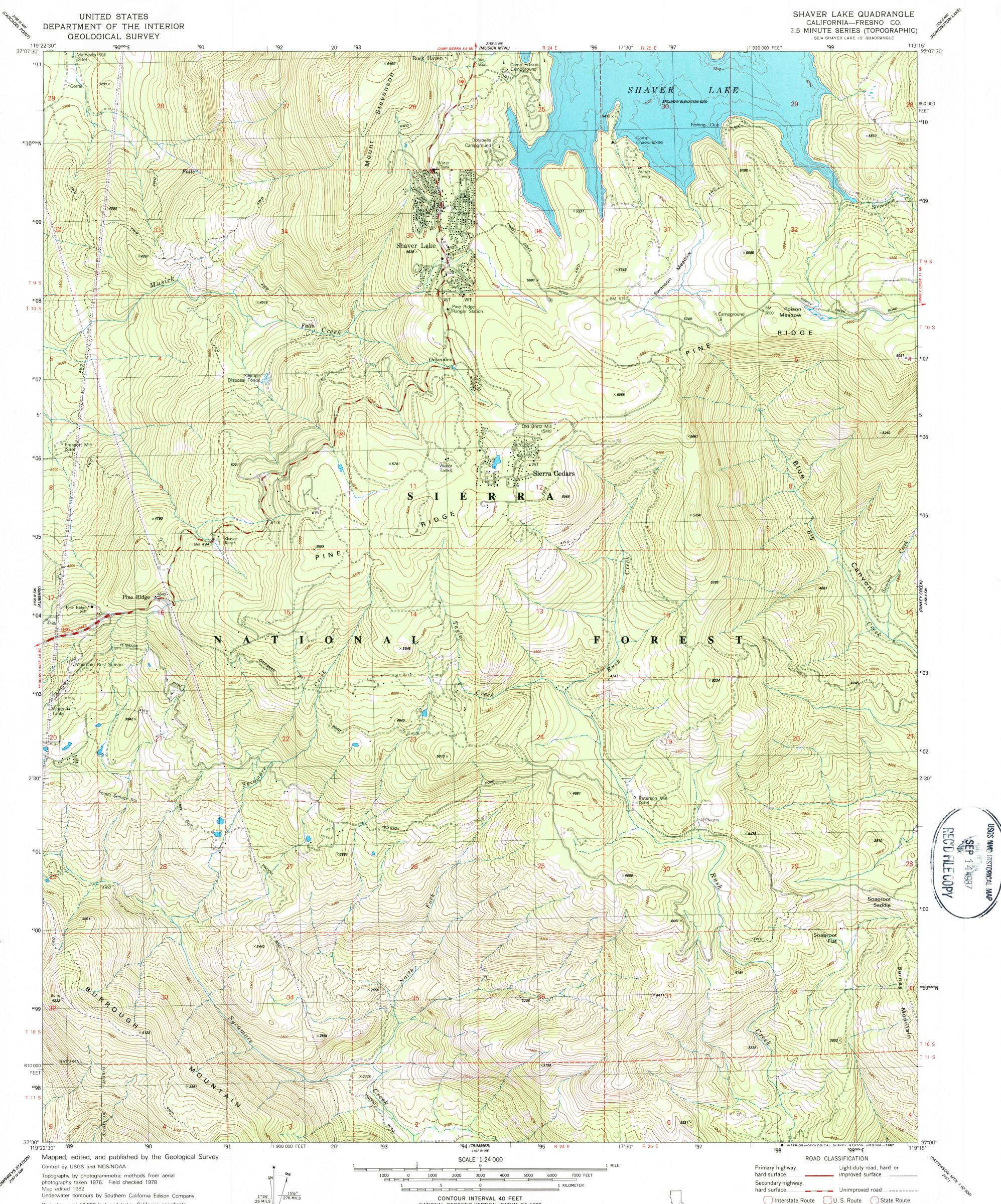
Projection and 10,000-foot grid ticks: California coordinate system, zone 4 (Lambert conformal conic) 1000-meter Universal Transverse Mercator grid, zone 11 1927 North American Datum To place on the predicted North American Datum 1983 move the projection lines 9 meters north and 86 meters east as shown by dashed corner ticks
