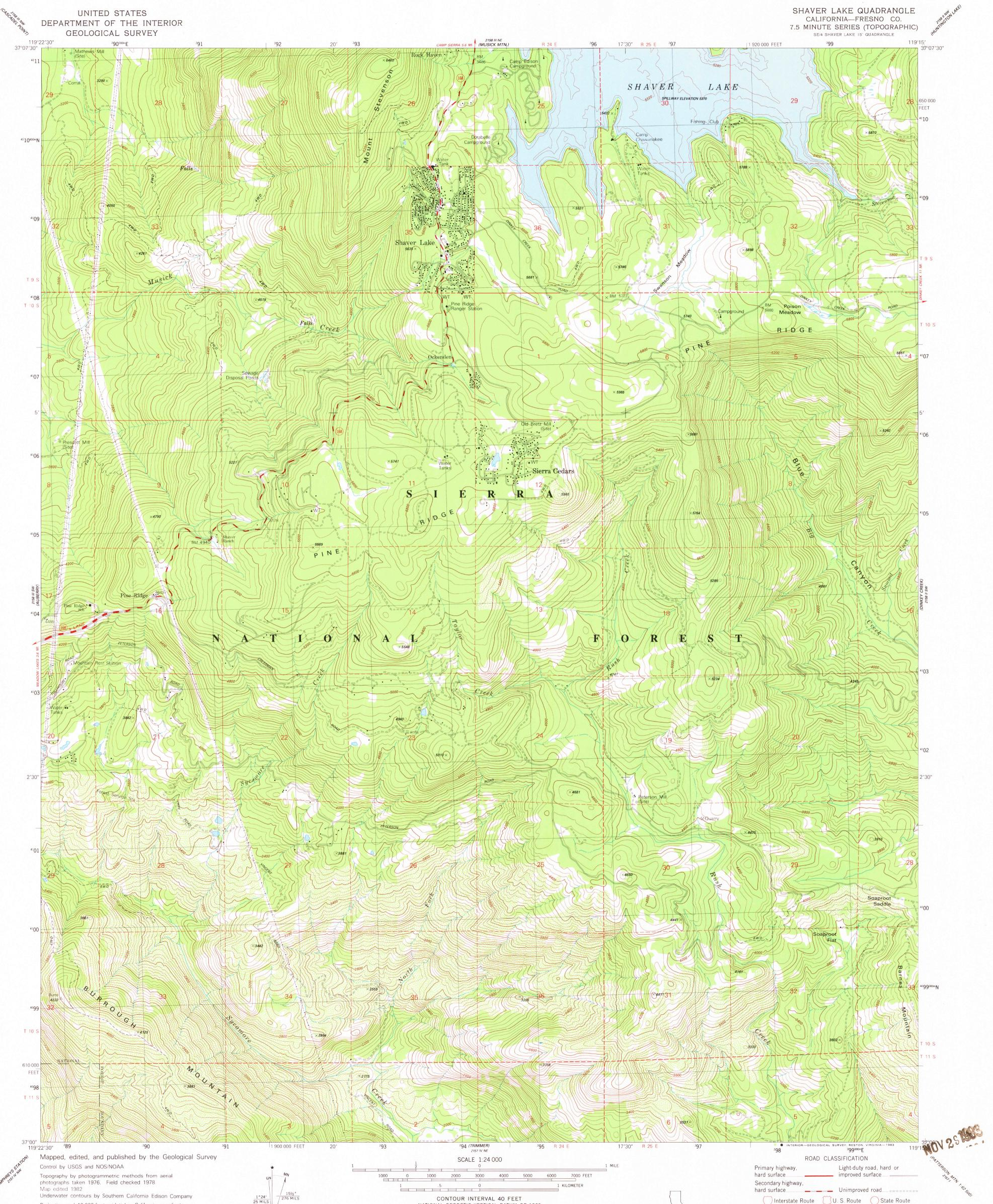
Projection and 10,000-foot grid ticks: California coordinate system, zone 4 (Lambert conformal conic) 1000-meter Universal Transverse Mercator grid, zone 11 1927 North American Datum To place on the predicted North American Datum 1983 move the projection lines 9 meters north and 86 meters east as shown by dashed corner ticks There may be private inholdings within the boundaries of the National or State reservations shown on this map
