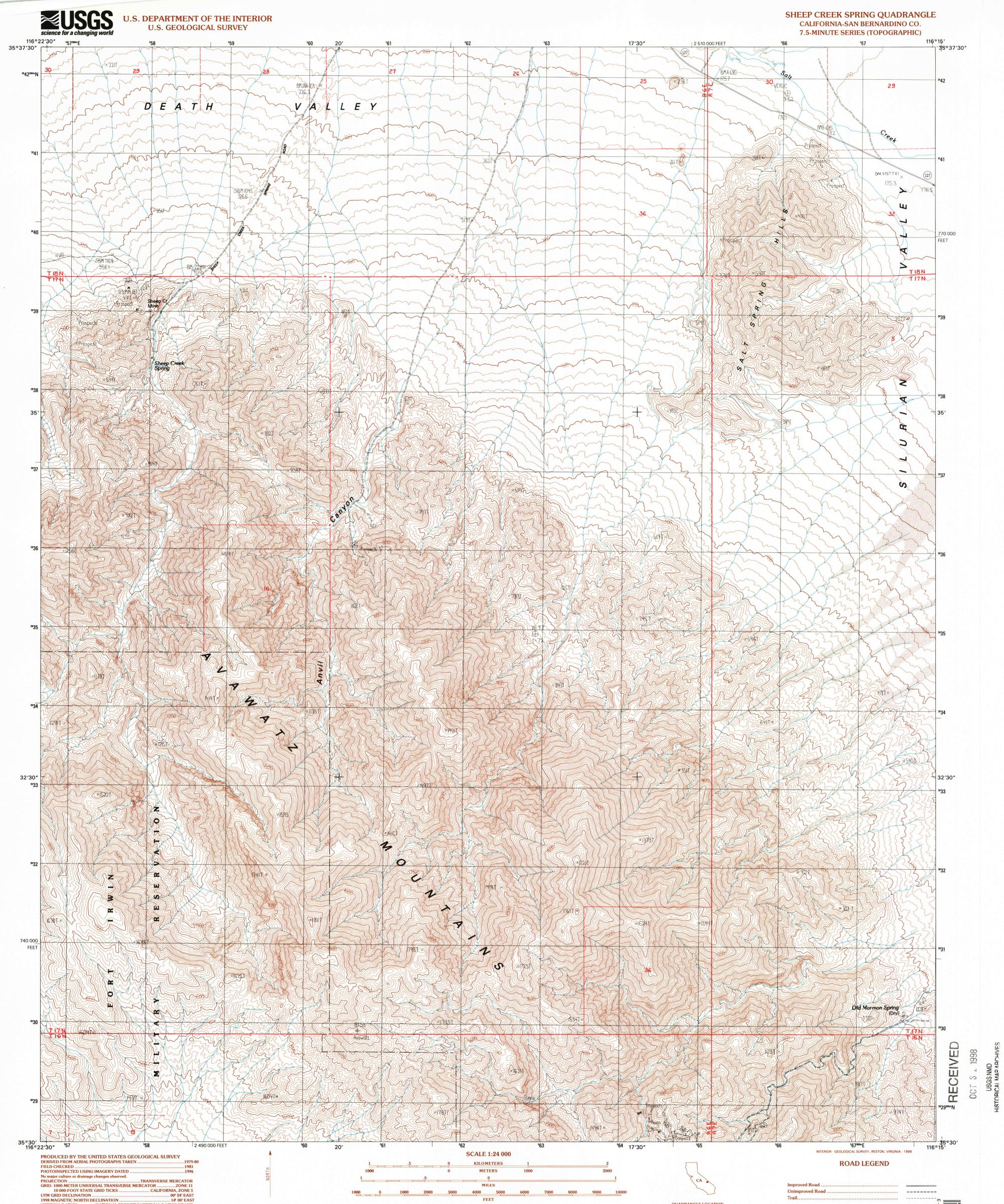
PROVISIONAL MAP Produced from original manuscript drawings. Information shown as of date of field check. 2 CONTOUR INTERVAL 10 METERS NATIONAL GEODETIC VERTICAL DATUM OF 1929 TO CONVERT FROM METERS TO FEET, MULTIPLY BY 3.2808
