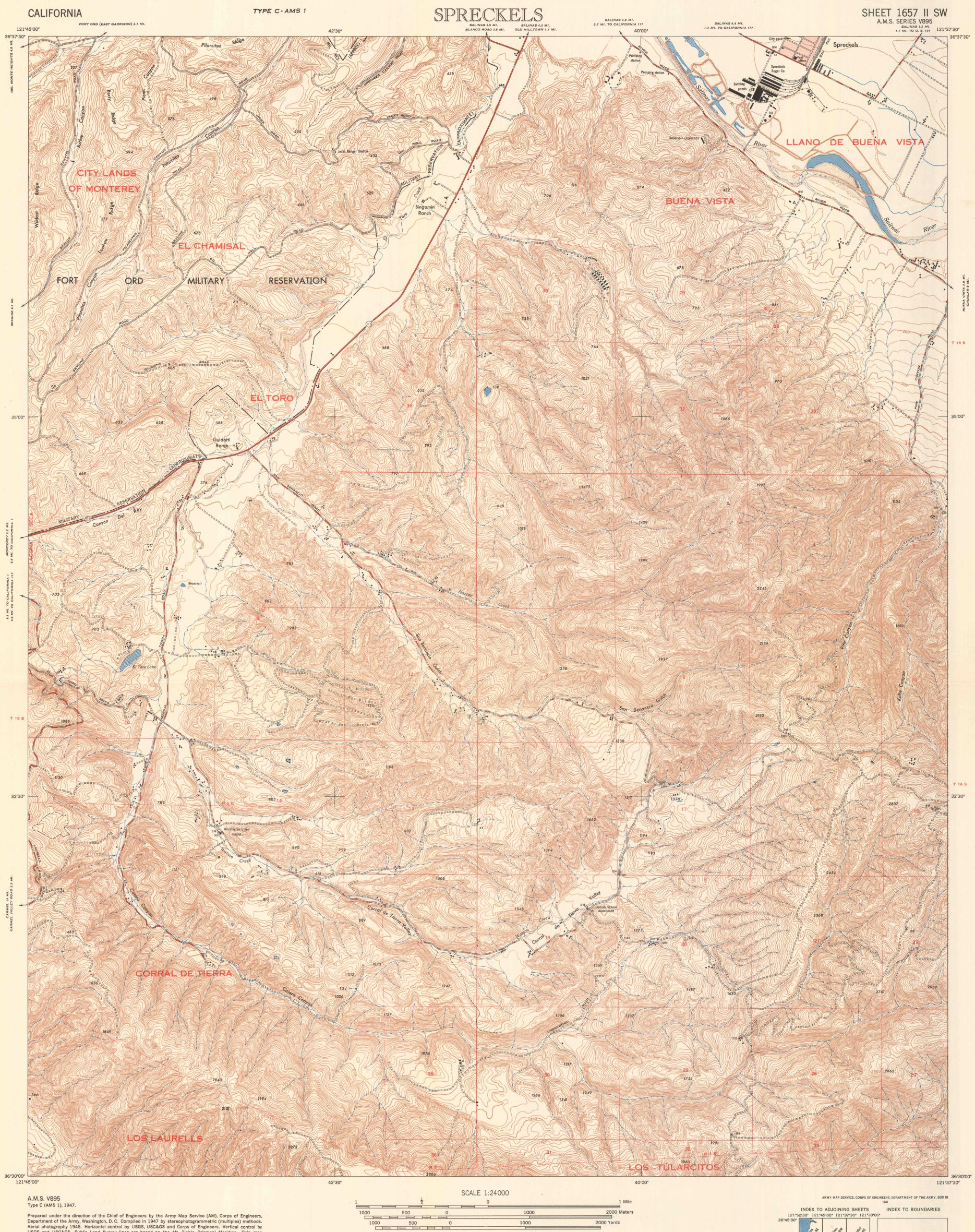
Prepared under the direction of the Chief of Engineers by the Army Map Service (AM), Corps of Engineers, Department of the Army, Washington, D. C. Compiled in 1947 by stereophotogrammetric (multiplex) methods. Aerial photography 1945. Horizontal control by USGS, USC&GS and Corps of Engineers. Vertical control by USGS and USC&GS. Public Land Survey lines are based on the Mt. Diablo Principal Meridian. This map complies with the national standard map accuracy requirements. Map field checked.
