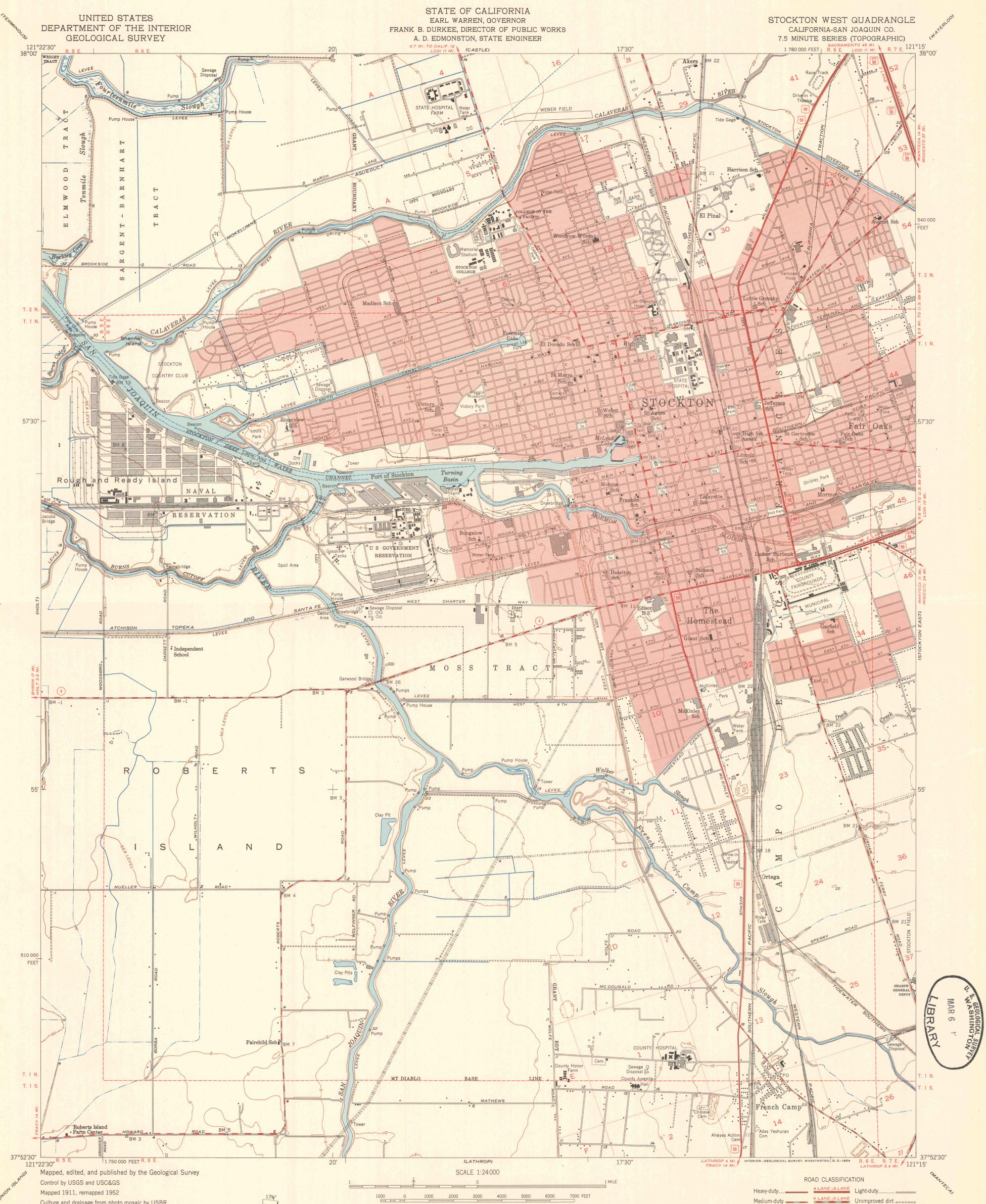
Culture and drainage from photo mosaic by USBR Aerial photographs taken 1949 Topography from plane-table surveys by USGS 1952 Hydrography from USC&GS chart 5527 Polyconic projection. 1927 North American datum 10,000-foot grid based on California coordinate system, zone 3 Red tint indicates areas in which only landmark buildings are shown Dashed land lines indicate approximate locations Dotted land lines were established by private survey
