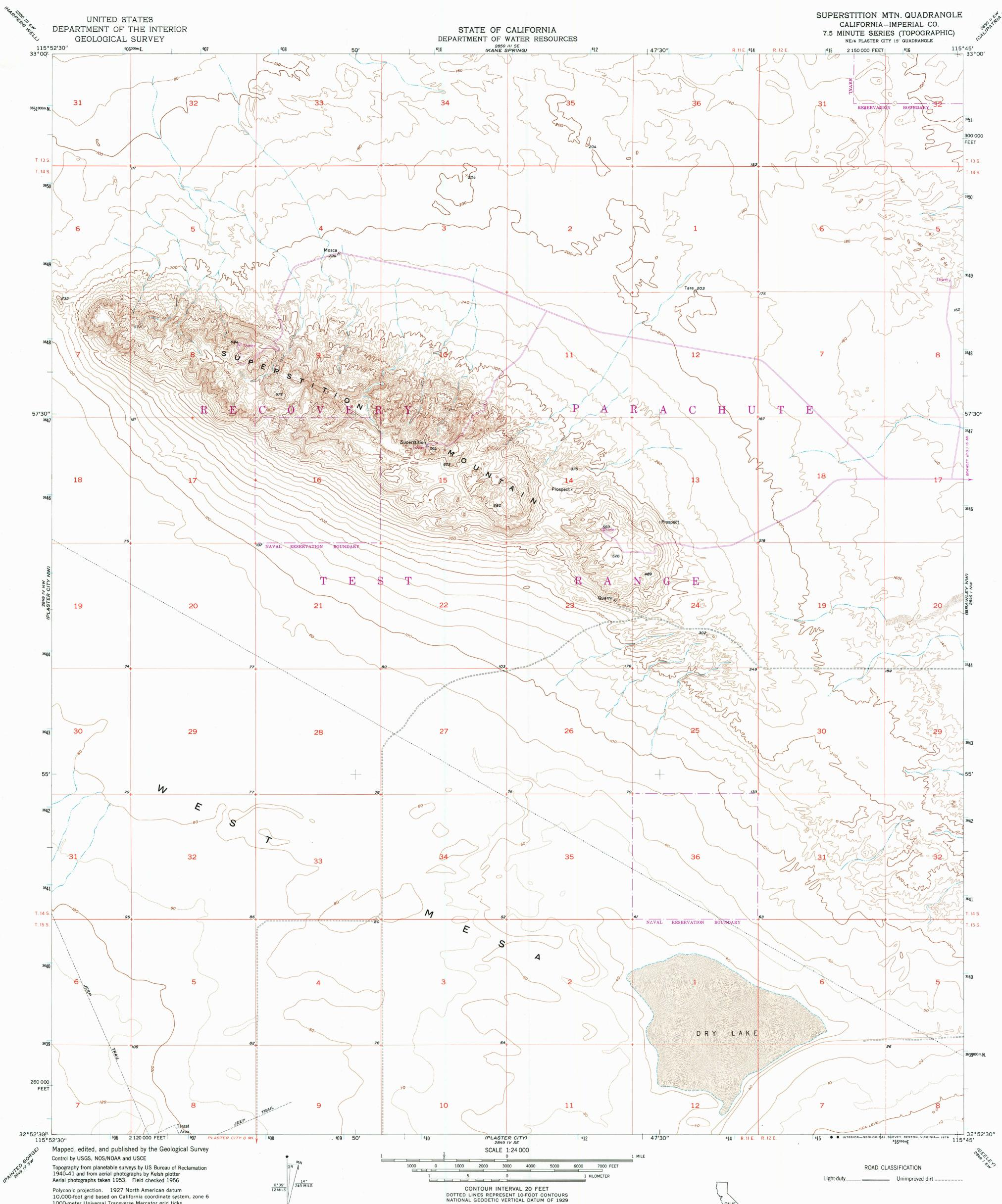
Polyconic projection. 1927 North American datum 10,000-foot grid based on California coordinate system, zone 6 1000-meter Universal Transverse Mercator grid ticks, zone 11, shown in blue To place on the predicted North American Datum 1983, move the projection lines 3 meters south and 77 meters west as shown by dashed corner ticks There may be private inholdings within the boundaries of the National or State reservations shown on this map
