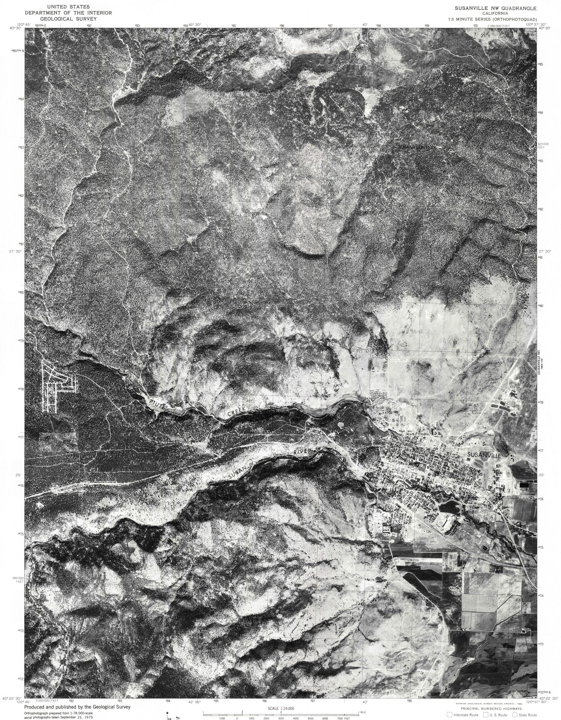
Projection and 10,000-foot grid ticks: California coordinate system, zone 1 (Lambert conformal conic) 1000-meter Universal Transverse Mercator grid ticks, zone 10. 1927 North American datum
