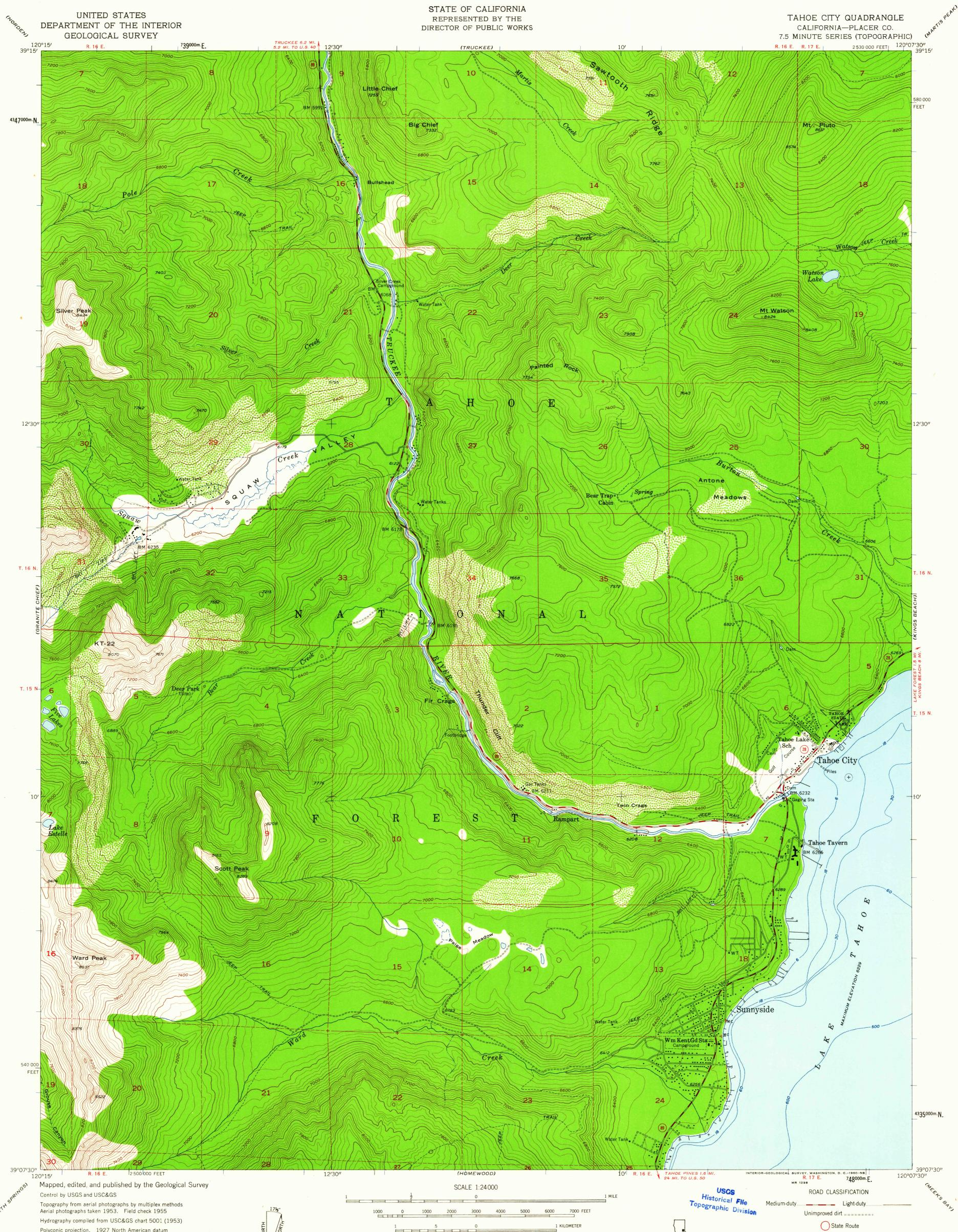
Polyconic projection. 1927 North American datum 10,000-foot grid based on California coordinate system, zone 2 Dashed land lines indicate approximate locations 1000-meter Universal Transverse Mercator grid ticks, zone 10, shown in blue
