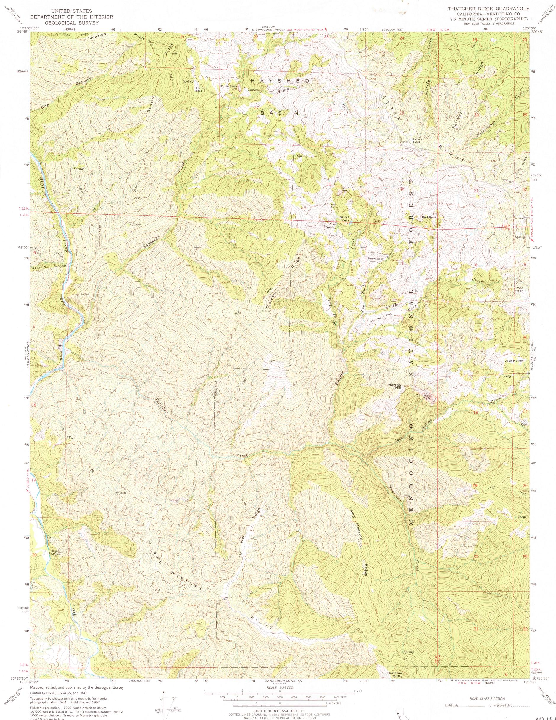
10,000-foot grid based on California coordinate system, zone 2 1000-meter Universal Transverse Mercator grid ticks, zone 10, shown in blue To place on the predicted North American Datum 1983 move the projection lines 18 meters north and 95 meters east as shown by dashed corner ticks
