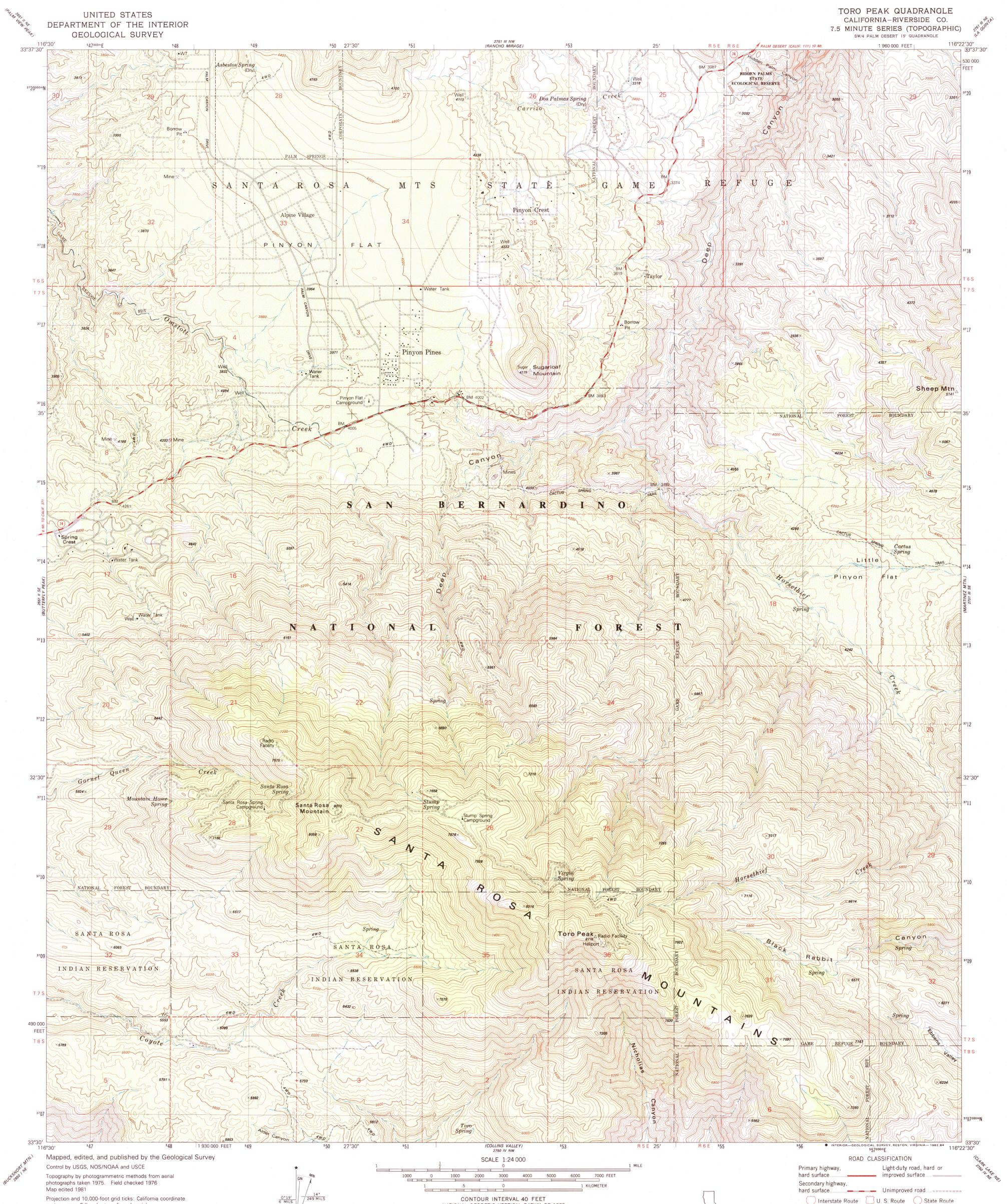
Projection and 10,000-root grid ticks: California coordinate system, zone 6 (Lambert conformal conic) 1000-meter Universal Transverse Mercator grid, zone 11 1927 North American Datum To place on the predicted North American Datum 1983 move the projection lines 1 meter south and 79 meters east as shown by dashed corner ticks There may be private inholdings within the boundaries of the National or State reservations shown on this map
