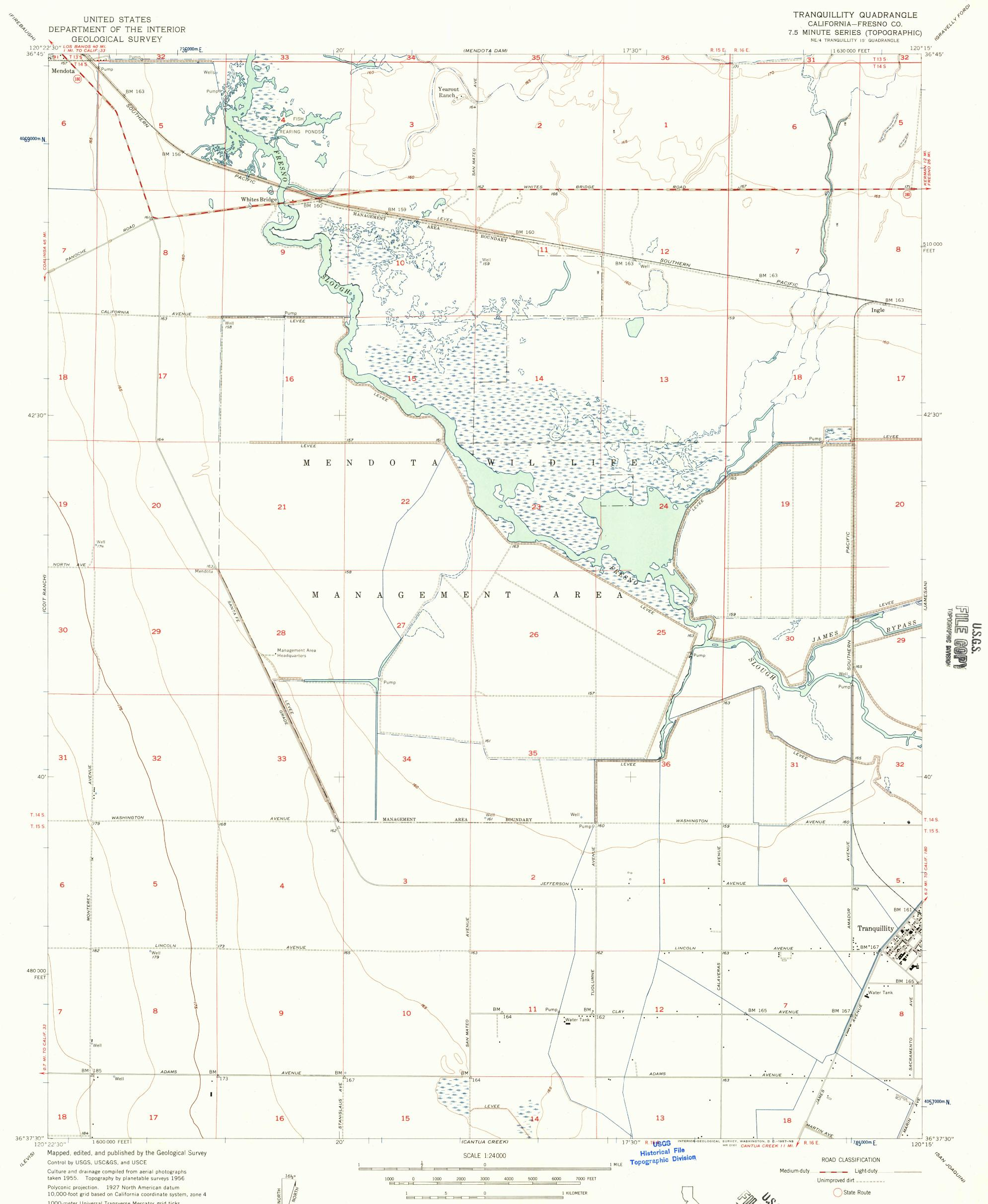
10,000-foot grid based on California coordinate system, zone 4 1000-meter Universal Transverse Mercator grid ticks, zone 10, shown in blue Dotted land lines were established by private surveys
