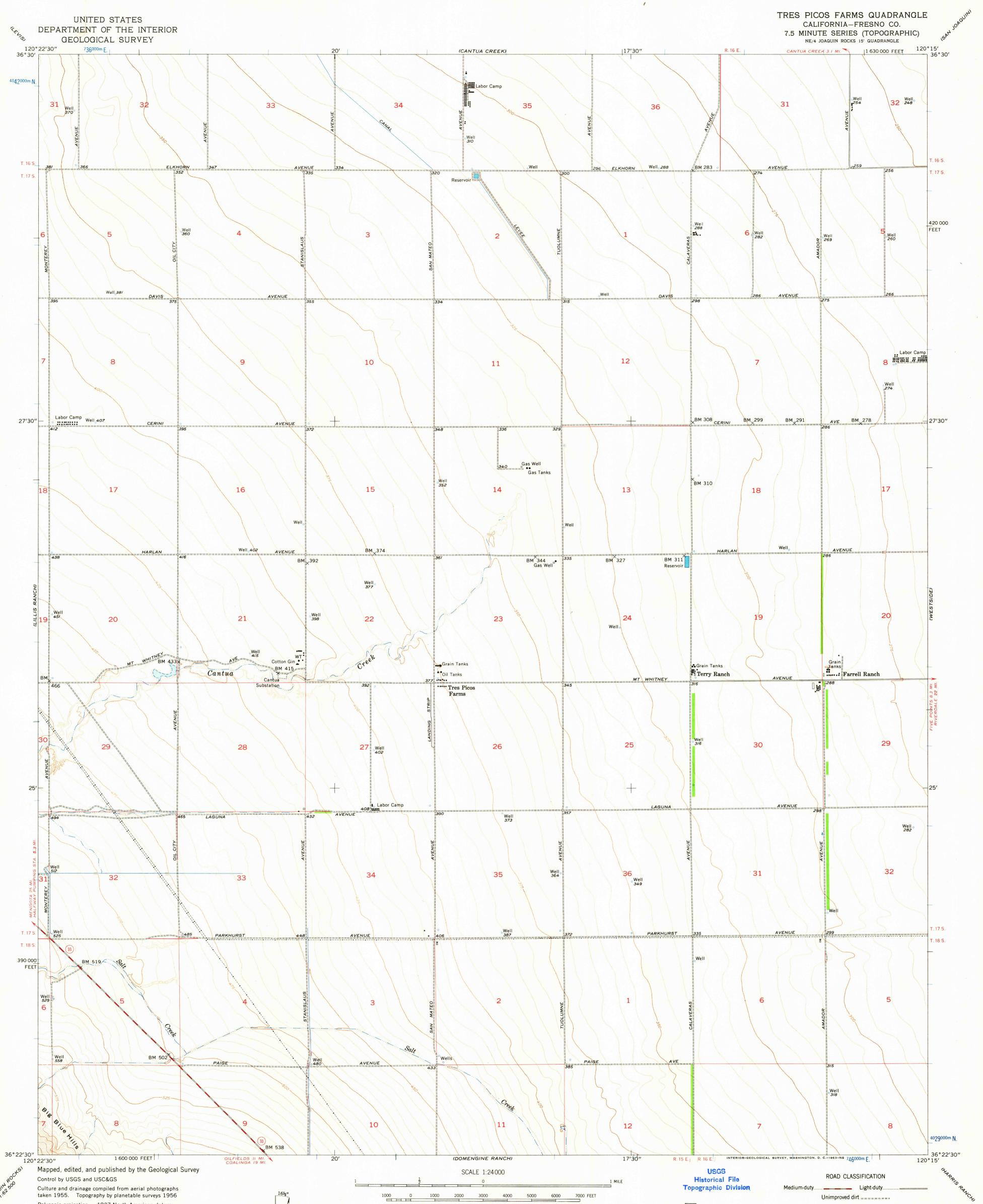
Polyconic projection. 1927 North American datum 10,000-foot grid based on California coordinate system, zone 4 1000-meter Universal Transverse Mercator grid ticks, zone 10, shown in blue This map lies within a subsidence area
