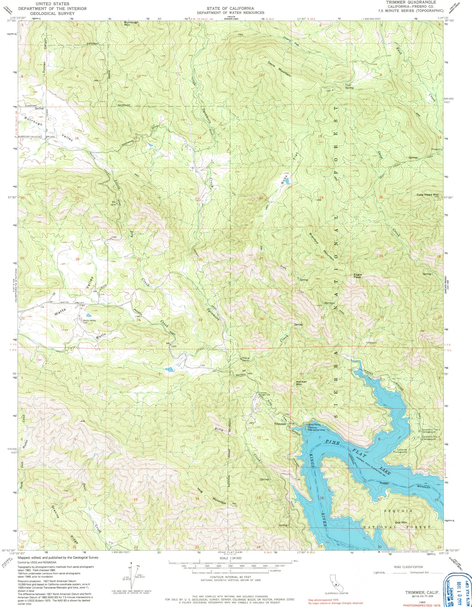
Polyconic projection. 1927 North American Datum 10,000-foot grid based on California coordinate system, zone 4 1000-meter Universal Transverse Mercator grid ticks, zone 11, shown in blue The difference between 1927 North American Datum and North American Datum of 1983 (NAD 83) for 7.5 minute intersections is given in USGS Bulletin 1875. The NAD 83 is shown by dashed corner ticks
