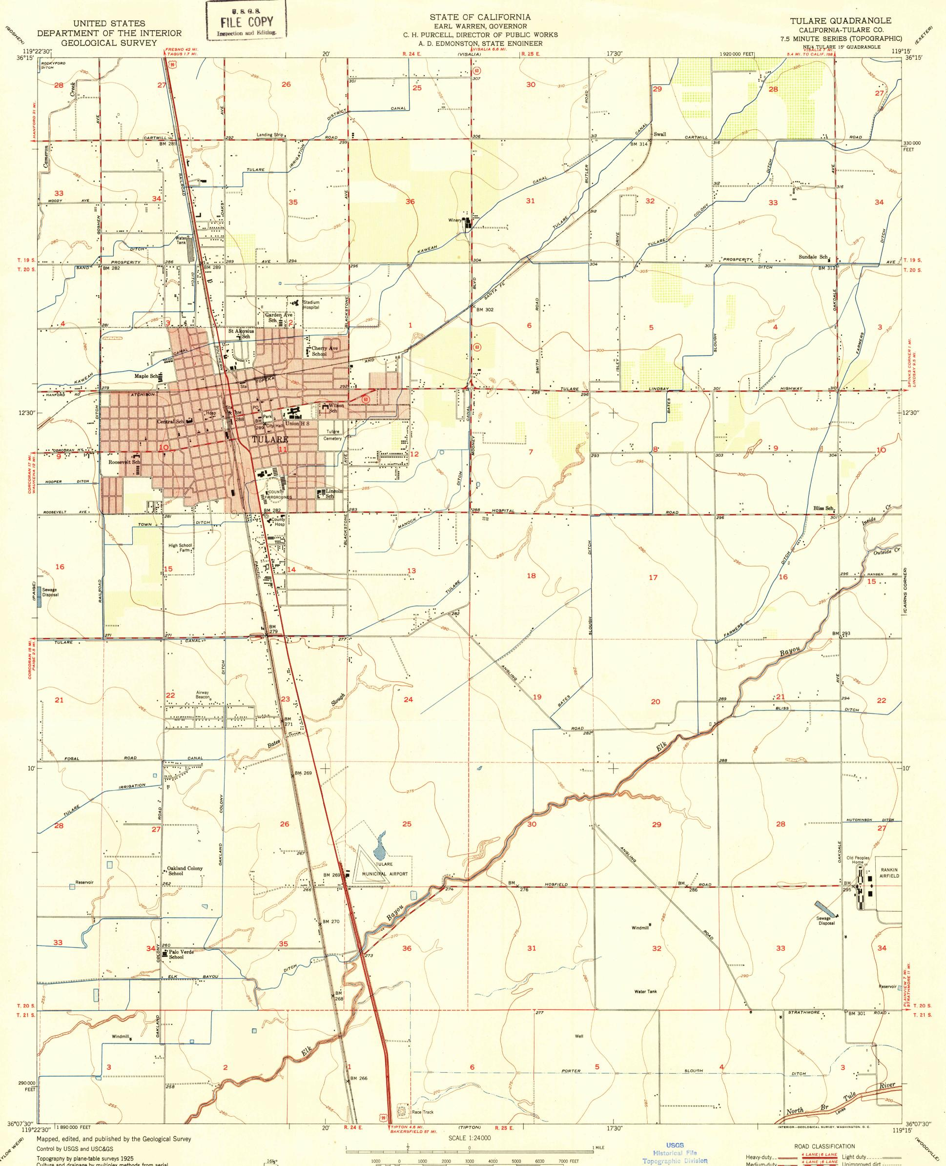
Culture and drainage by multiplex methods from aerial photographs taken 1946. Contour revision and field check 1950 Polyconic projection. 1927 North American datum 10,000-foot grid based on California coordinate system, zone 4 Red tint indicates area in which only landmark buildings are shown Dashed land lines indicate approximate location
