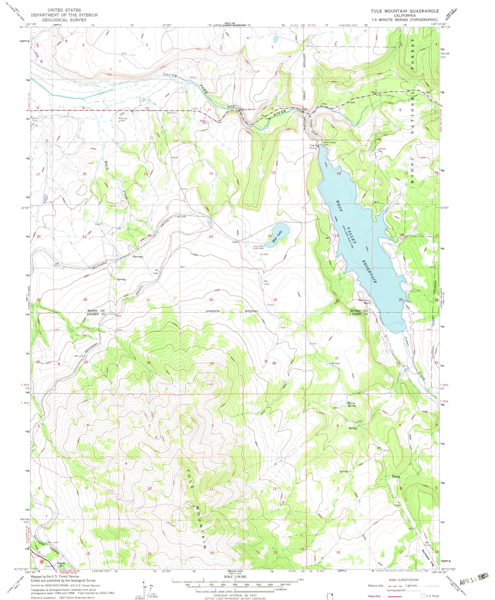
Polyconic projection. 1927 North American datum 10,000-foot grid based on California coordinate system, zone 1 1000-meter Universal Transverse Mercator grid ticks, zone 10, shown in blue
