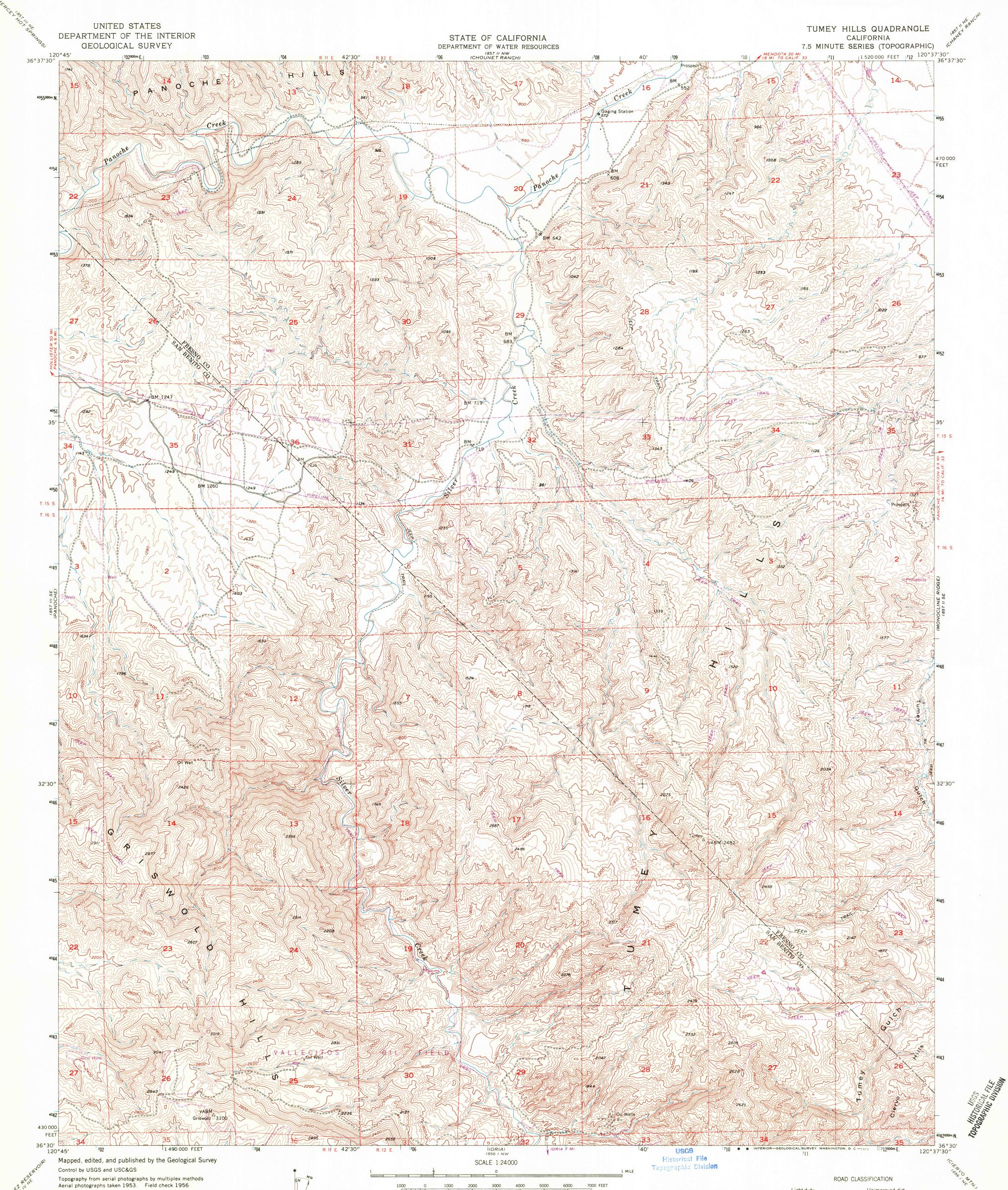
Polyconic projection. 1927 North American datum 10,000-foot grid based on California coordinate system, zone 4
