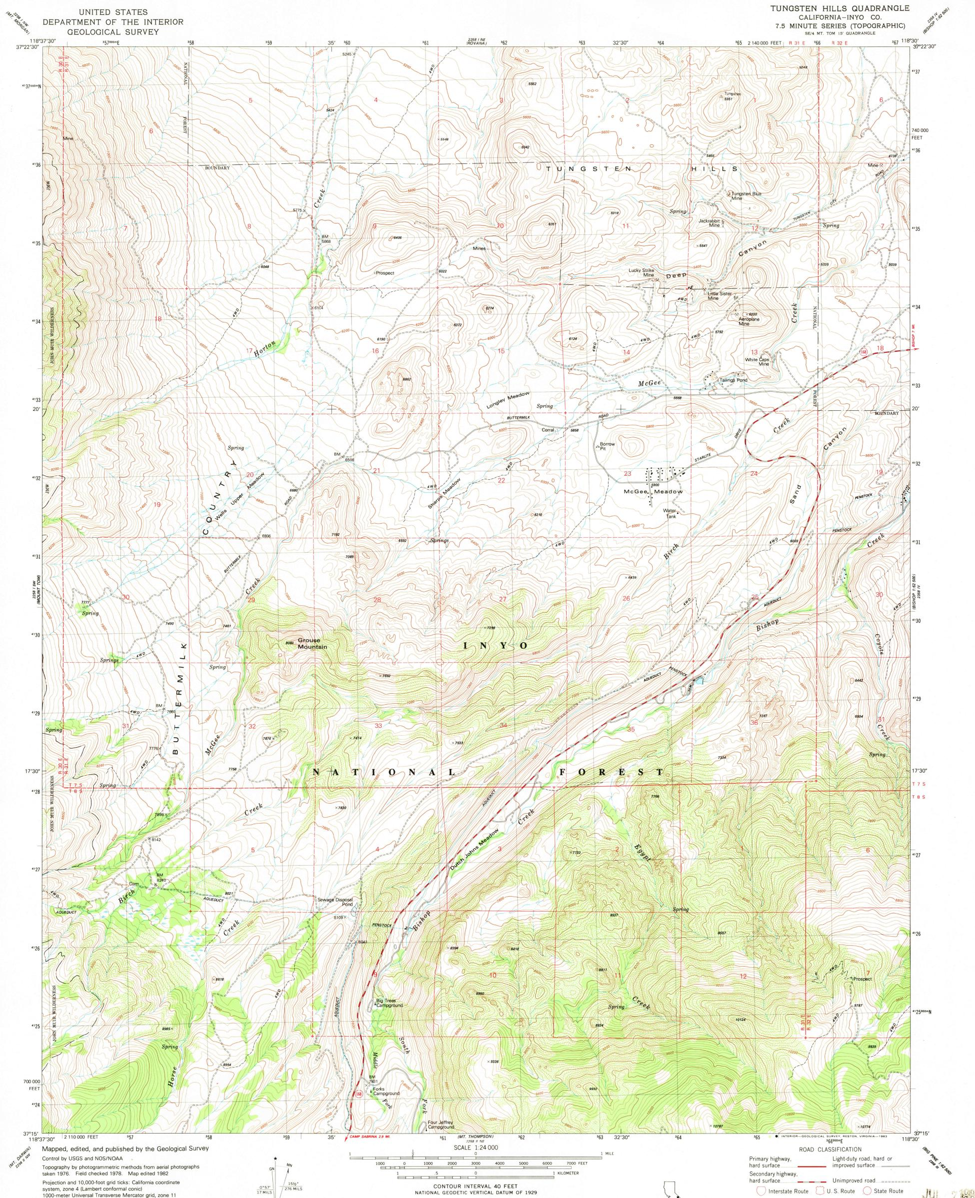
1000-meter Universal Transverse Mercator grid, zone 11 1927 North American Datum To place on the predicted North American Datum 1983 move the projection lines 10 meters north and 84 meters east as shown by dashed corner ticks
