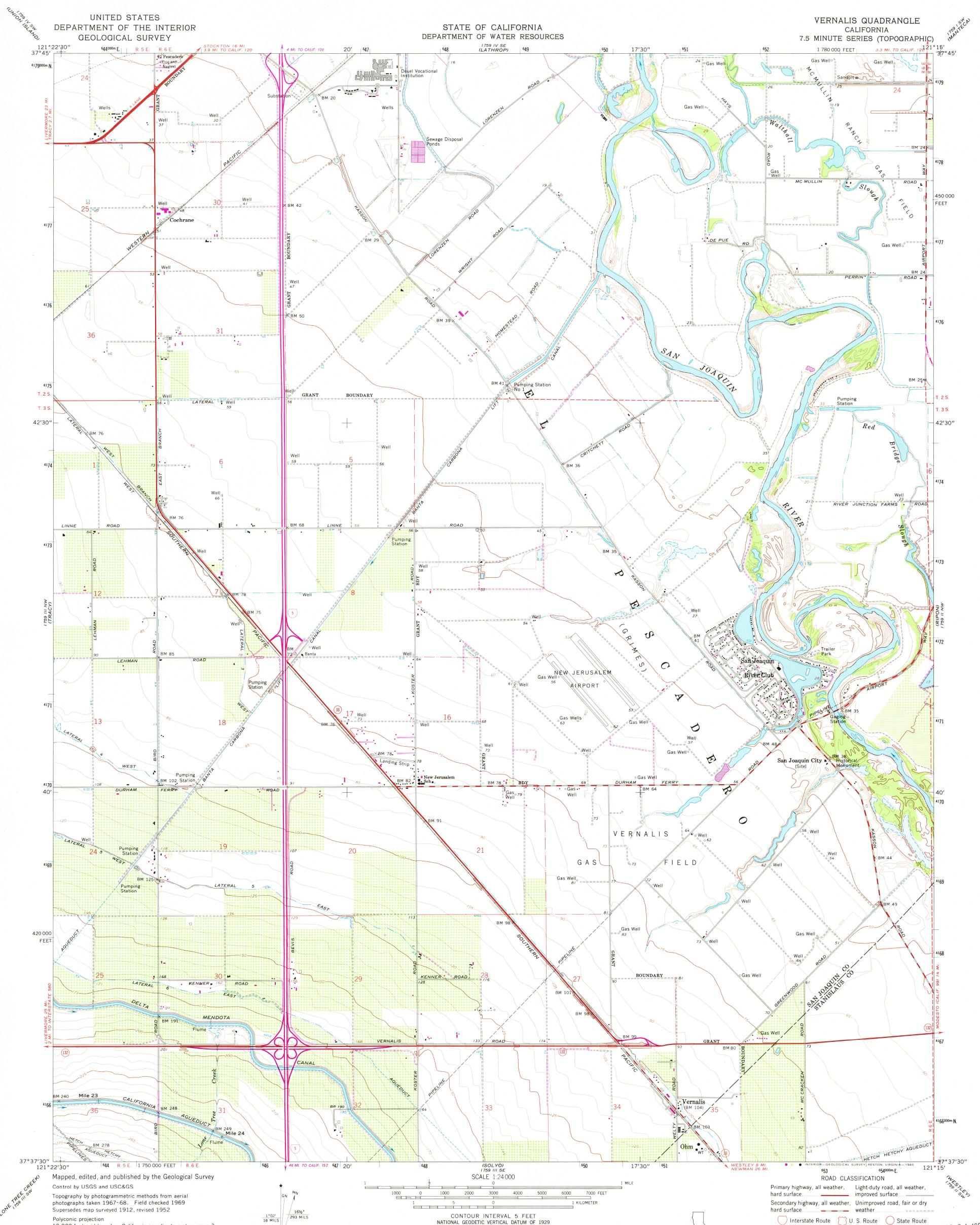
10,000-foot grid based on California coordinate system, zone 3 1000-meter Universal Transverse Mercator grid ticks, zone 10, shown in blue. 1927 North American Datum To place on the predicted North American Datum 1983 move the projection lines 12 meters north and 92 meters east as shown by dashed corner ticks
