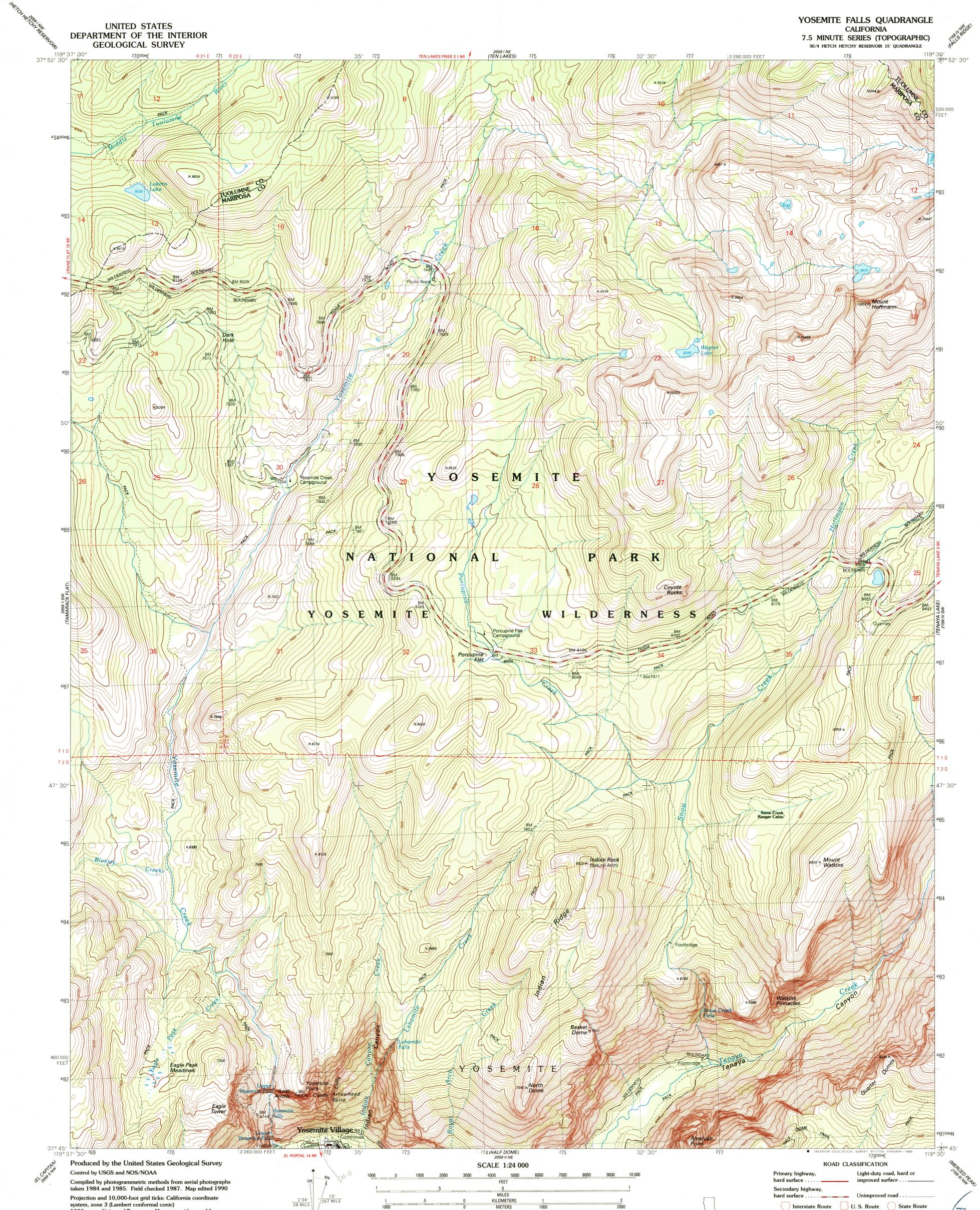
system, zone 3 (Lambert conformal conic) 1000-meter Universal Transverse Mercator grid, zone 11 1927 North American Datum To place on the predicted North American Datum 1983 move the projection lines 11 meters north and 87 meters east as shown by dashed corner ticks
