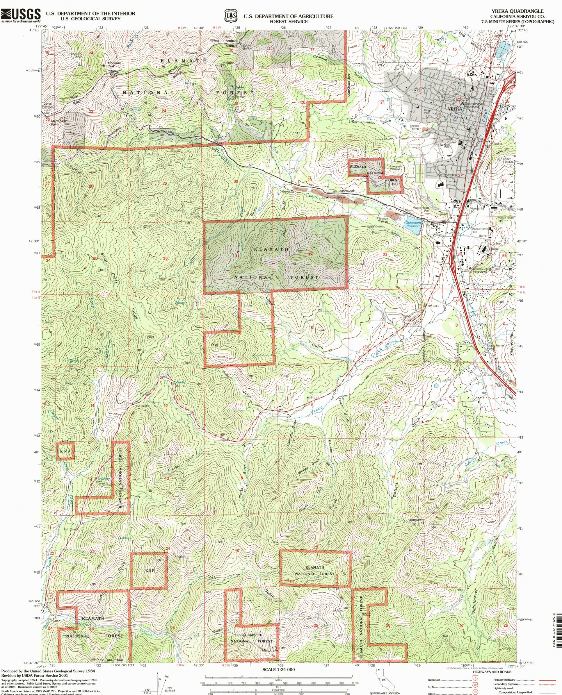
California coordinate system, zone 1 (Lambert conformal conic) Blue 1000-meter Universal Transverse Mercator ticks, zone 10
