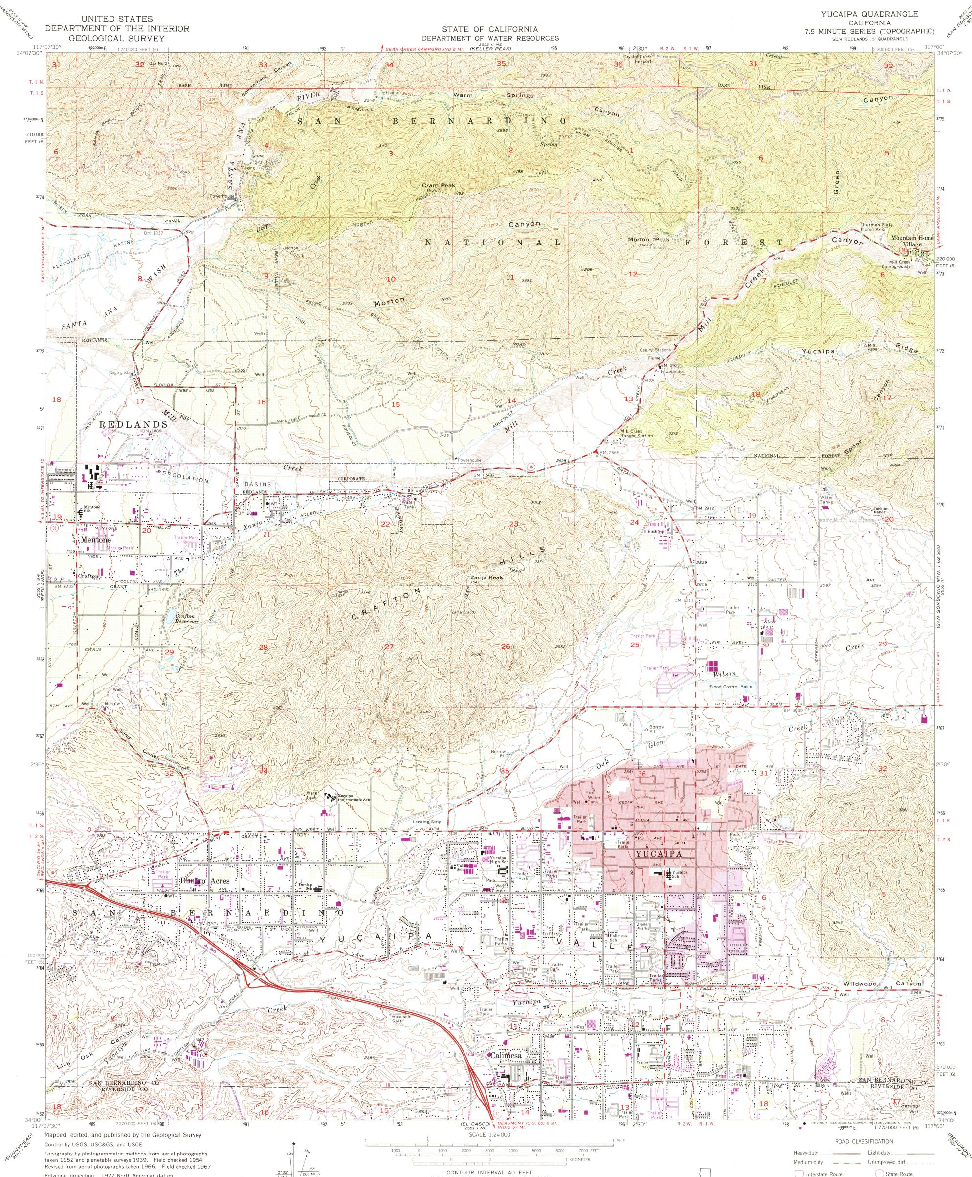
Polyconic projection. 1927 North American datum 10,000-foot grids based on California coordinate system, zones 5 and 6  $\,$ 1000-meter Universal Transverse Mercator grid ticks, zone 11, shown in blue
