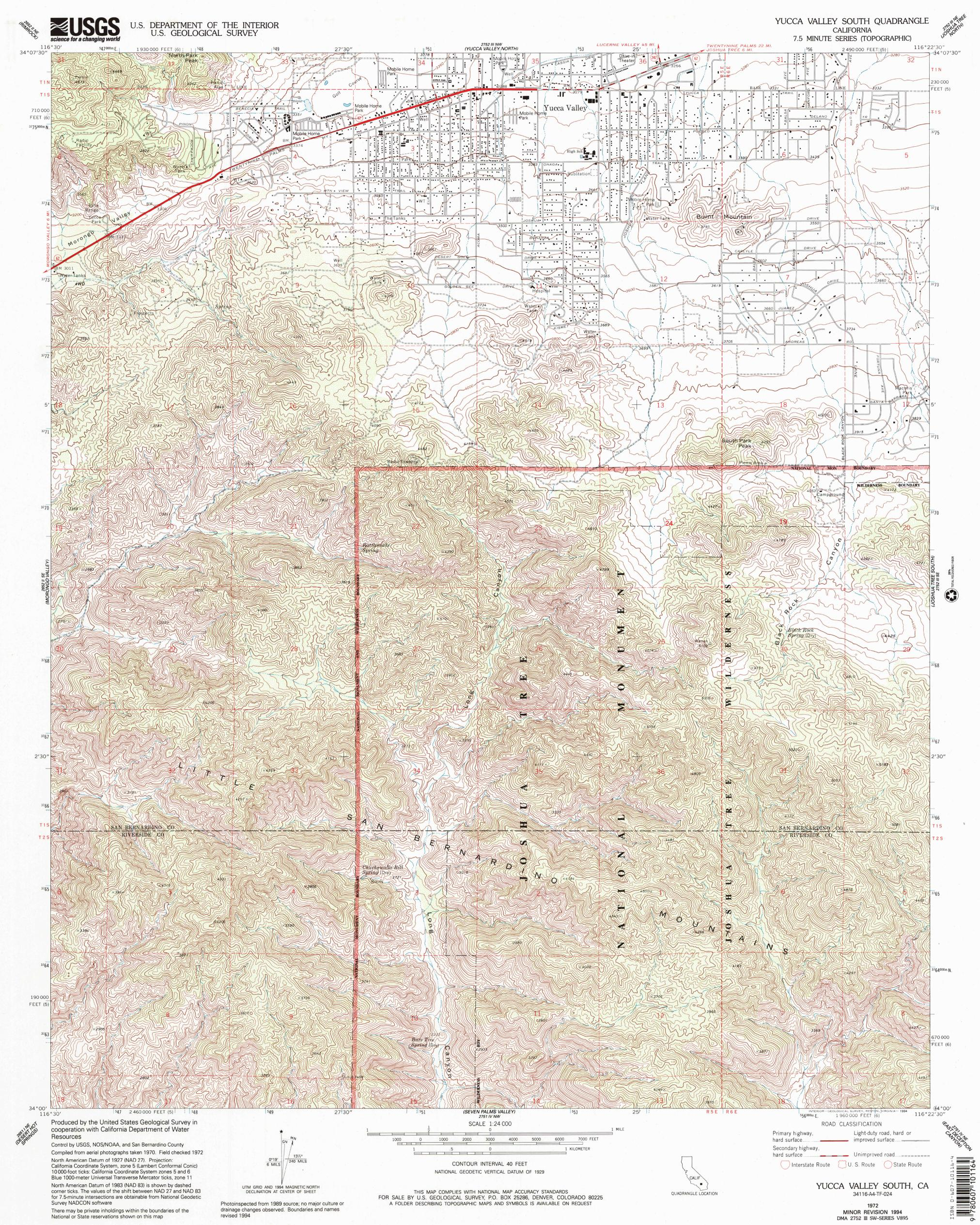
North American Datum of 1927 (NAD 27). Projection: California Coordinate System, zone 5 (Lambert Conformal Conic) 10 000-foot ticks: California Coordinate System zones 5 and 6 Blue 1000-meter Universal Transverse Mercator ticks, zone 11
