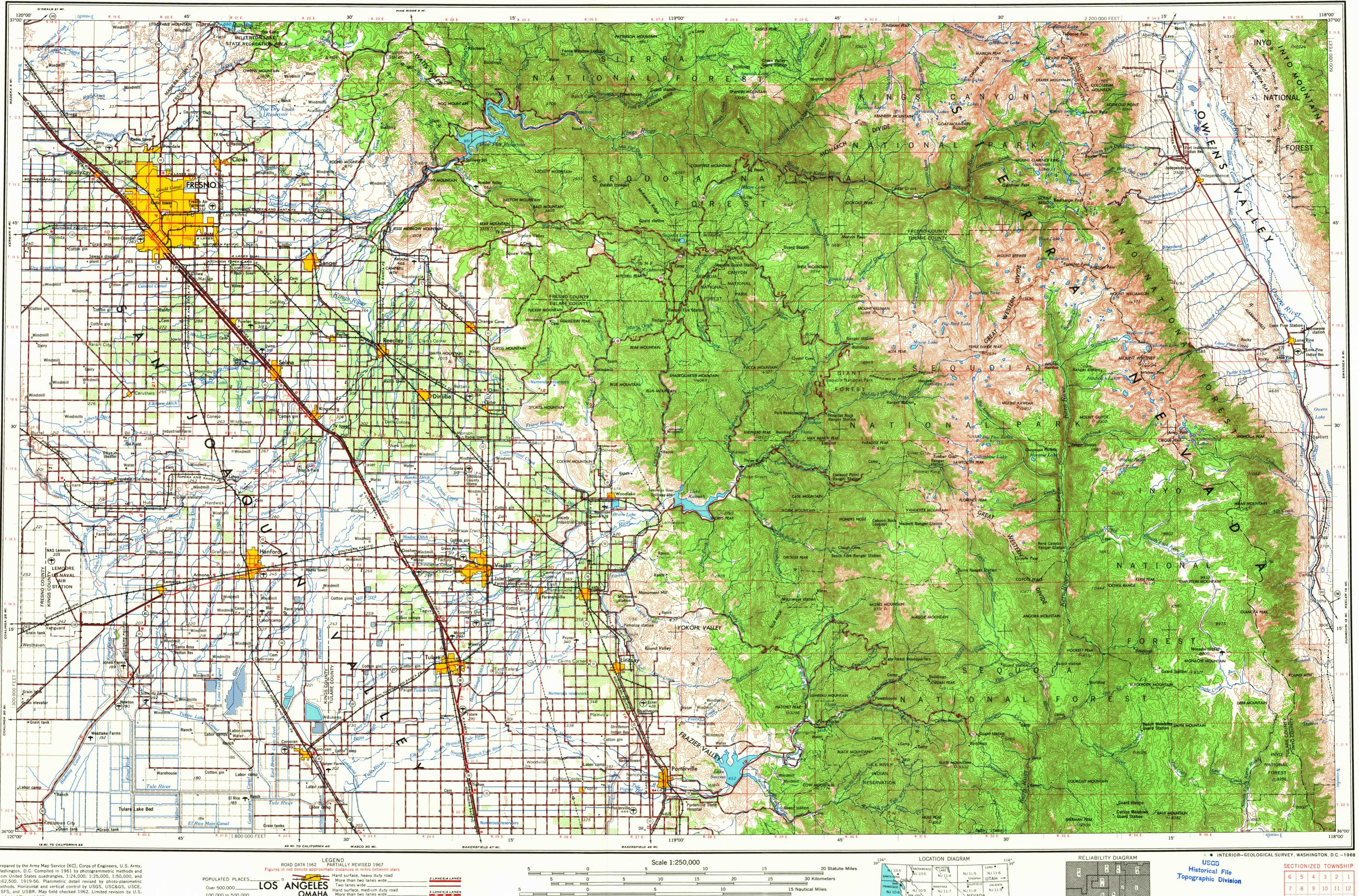
Prepared by the Army Map Service (KC), Corps of Engineers, U.S. Army, Washington, D.C. Compiled in 1961 by photogrammetric methods and from United States quadrangles, 1:24,000, 1:25,000, 1:50,000, and 1:62,500, 1919-56. Planimetric detail revised by photo-planimetric methods. Horizontal and vertical control by USGS, USC&GS, USCE, USFS, and USBR. Map field checked 1962. Limited revision by U.S.
