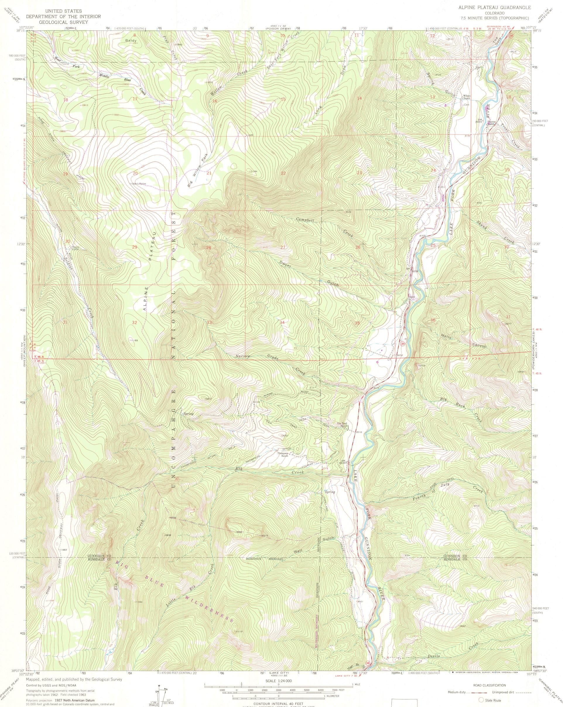
10,000-foot grids based on Colorado coordinate system, central and south zones 1000-meter Universal Transverse Mercator grid ticks, zone 13, shown in blue Certain land lines are omitted because of insufficient data To place on the predicted North American Datum 1983 move the projection lines 4 meters north and 54 meters east as shown by dashed corner ticks
