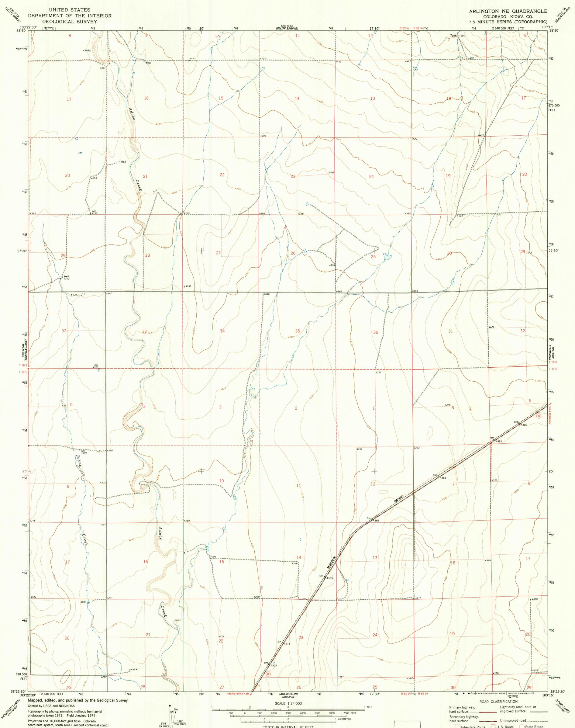
coordinate system, south zone (Lambert conformal conic, 1000-meter Universal Transverse Mercator grid ticks, zone 13, shown in blue. 1927 North American datum Fine red dashed lines indicate selected fence lines
