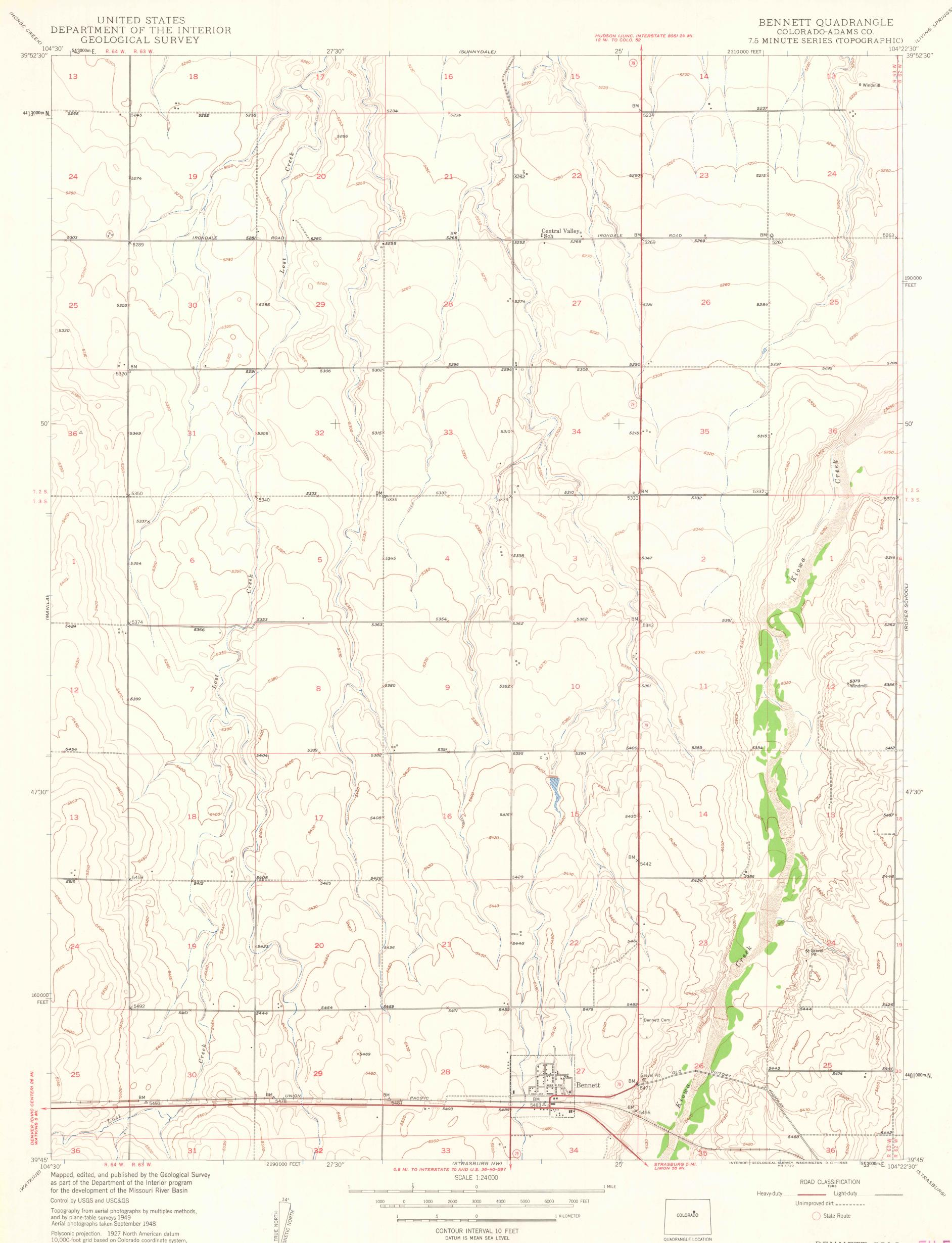
Topography from aerial photographs by multiplex methods, and by plane-table surveys 1949 Aerial photographs taken September 1948 Polyconic projection. 1927 North American datum 10,000-foot grid based on Colorado coordinate system, north zone 1000-meter Universal Transverse Mercator grid ticks, zone 13, shown in blue
