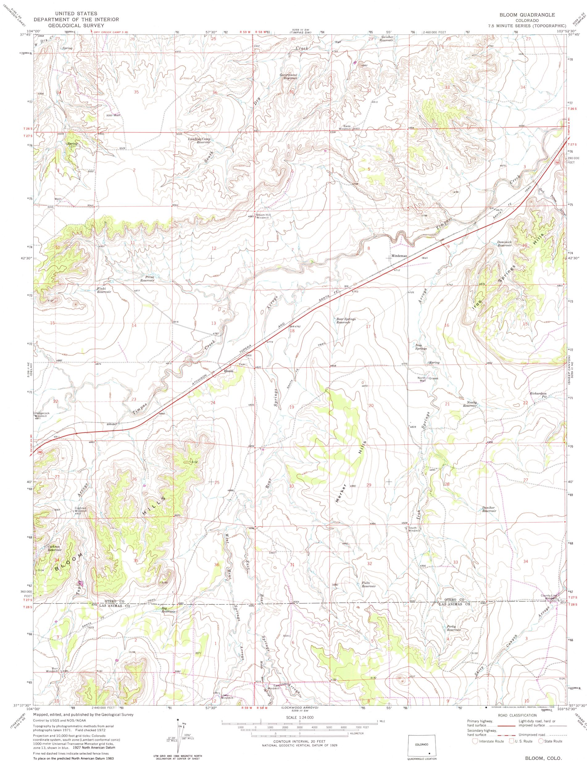
To place on the predicted North American Datum 1983 move the projection lines 2 meters north and 45 meters east as shown by dashed corner ticks
