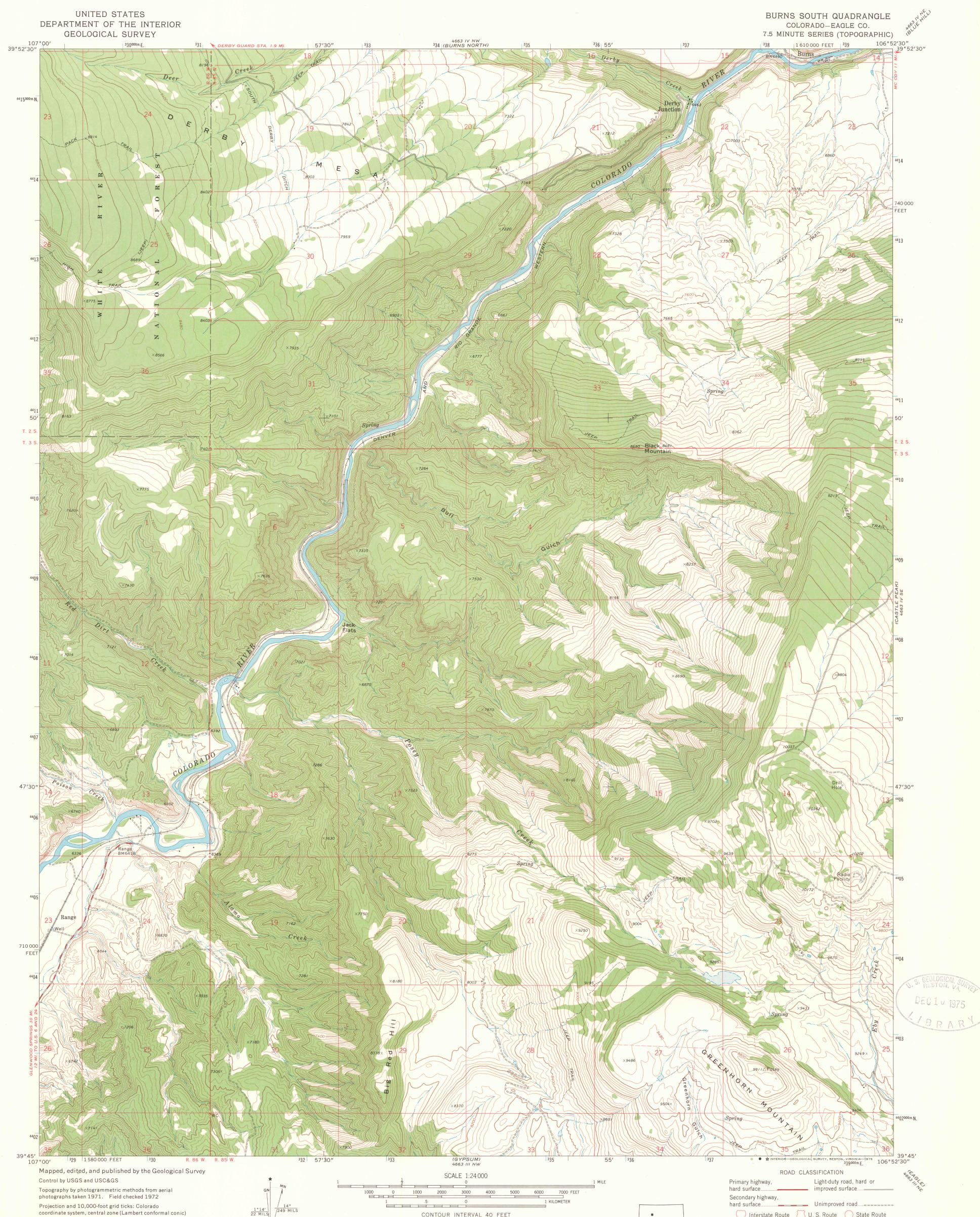
coordinate system, central zone (Lambert conformal conic) 1000-meter Universal Transverse Mercator grid ticks, zone 13, shown in blue. 1927 North American datum
